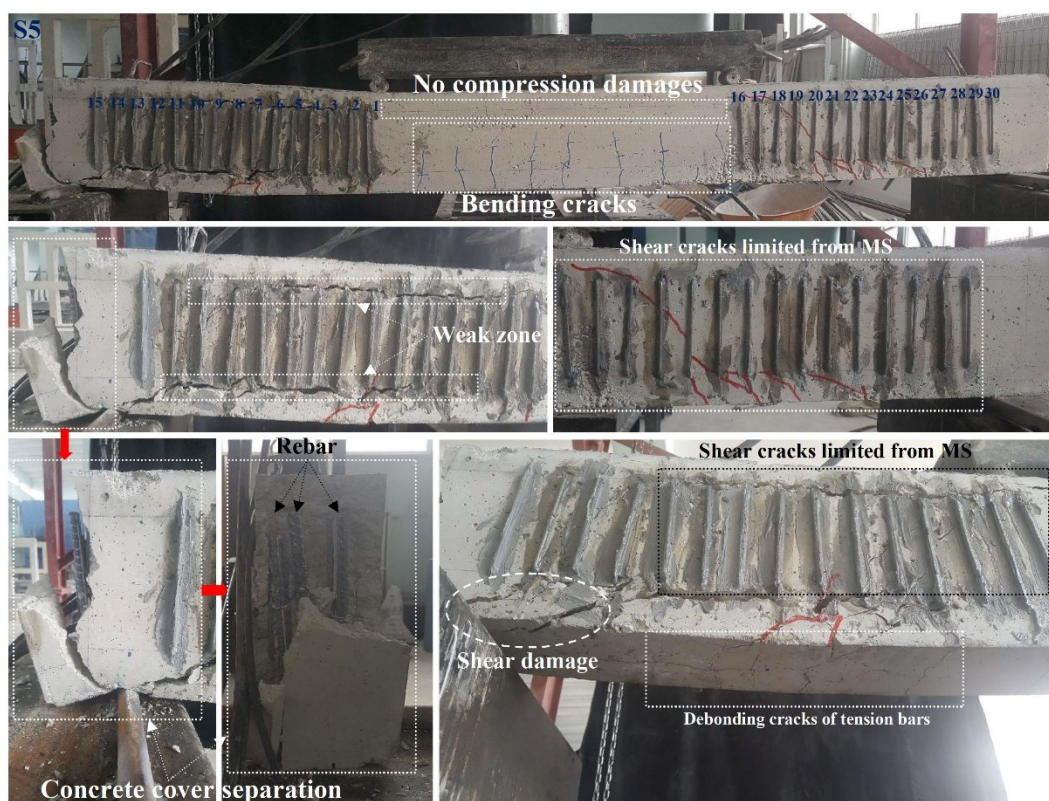
Figure 12. Damages at S5.
