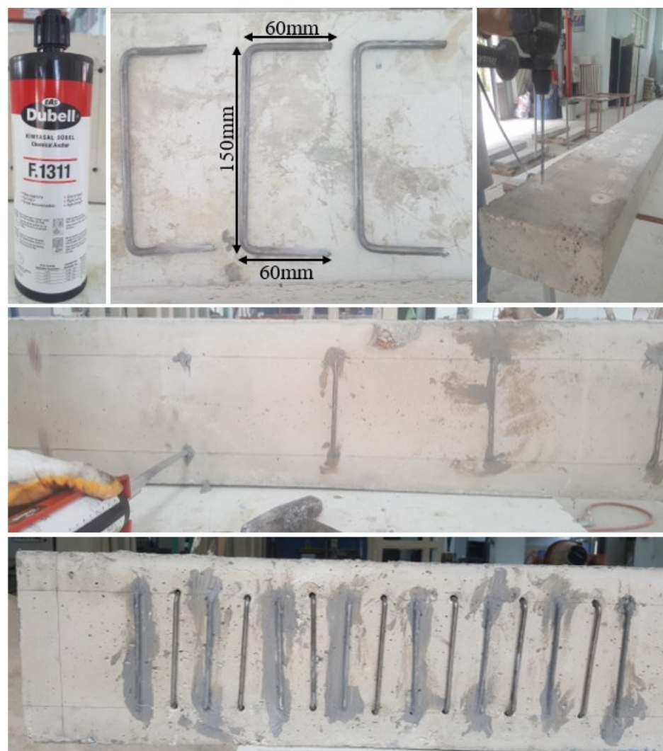
Figure 2. Strengthening beams with MSS.
