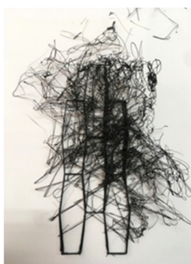
Figure 22. Pyramidal base failures due to inadequate 3D printing settings.
