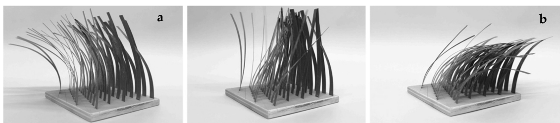
Figure 10. Recycled package paper and Kapton tape and their shape change influenced by temperature variations, 18 °C (a) up to 50 °C (b), 7 row arrangement of the lamellae.
