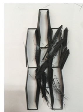
Figure 22. Pyramidal base failures due to inadequate 3D printing settings.
