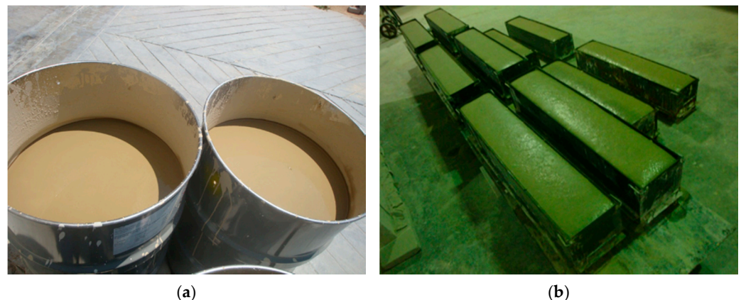
Figure 1. Mixture of AAC (a) and mixture of AAC in the mold for the autoclaving process (b).
