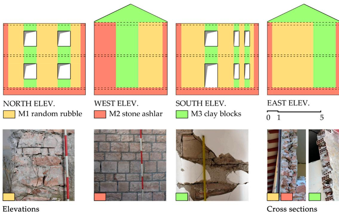
**Figure 5.** Distribution of masonry types within IACP building.
