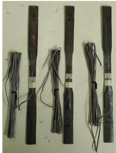
**Figure 7.** Specimens with strain gauges for testing the elastic modulus.
