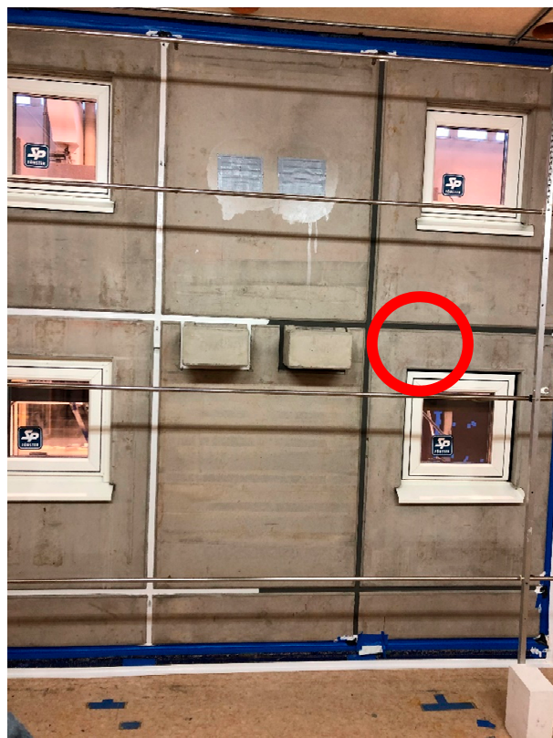
Figure 8. Laboratory concrete facade test setup, where the red circle marks the studied point A19 [19].
