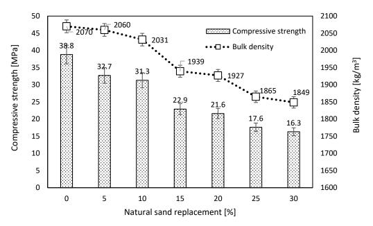
Figure 5. Compressive strength and bulk density after 28 days.
