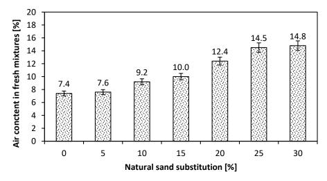
Figure 4. Content of air in fresh mixtures.
