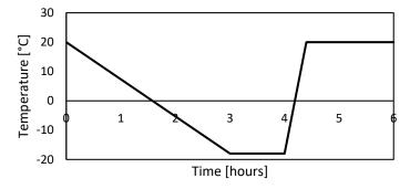
Figure 3. The regime of a freeze-thaw cycle.
