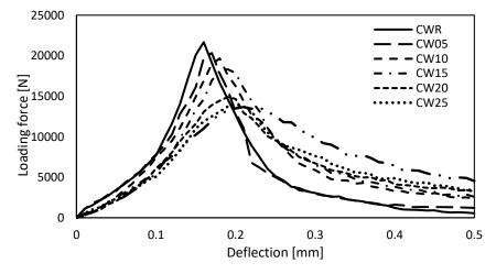
Figure 6. The records of flexural tests after 28 days.
