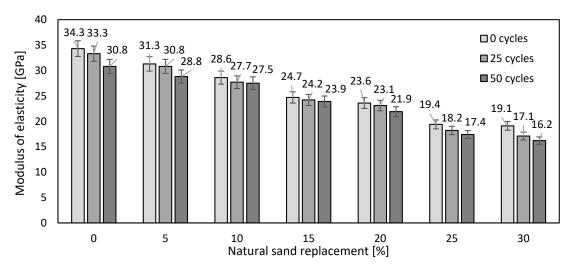
Figure 7. Dynamic modulus of elasticity during freezing-thawing.
