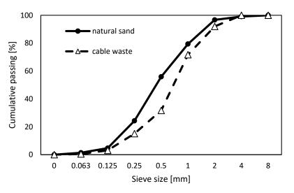
Figure 1. Cumulative passing of studied cable waste and replaced natural sand.
