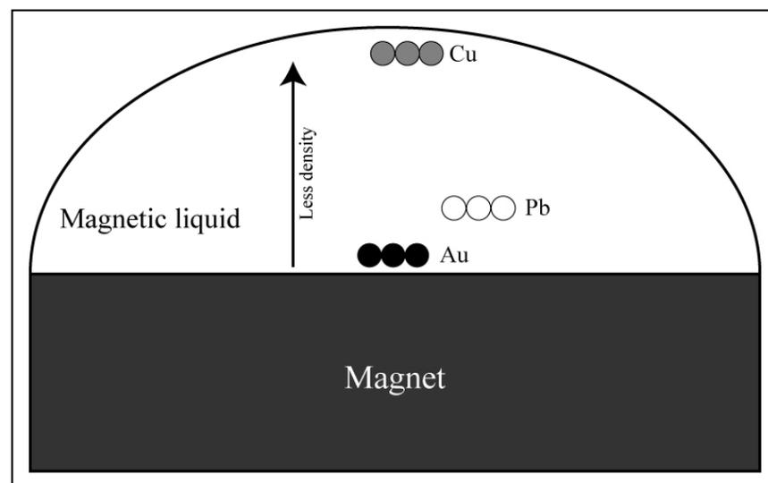
**Figure 2.** Principle of magnetic density separation, redrawn from [74].
