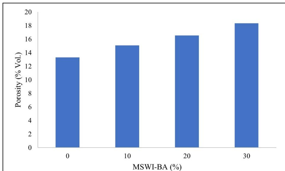
**Figure 8.** Porosity of concrete containing MSWI-BA, with data from [86].
