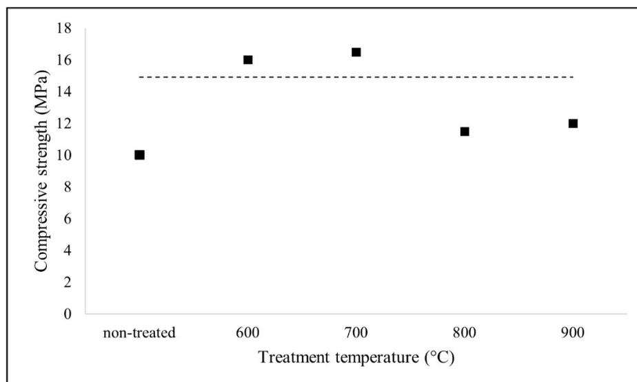
**Figure 6.** Effect of thermal treatment of MSWI-BA on the compressive strength of concrete at 28 days, redrawn from [90].
