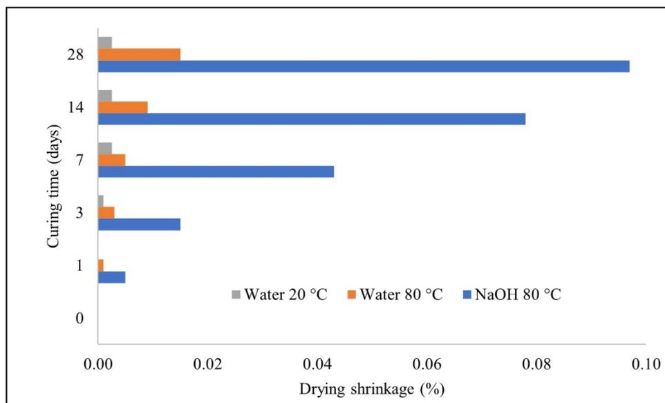
**Figure 9.** Drying shrinkage of dry-mixed cement mortar containing MSWI-BA, subjected to different curing regimes. Redrawn from [44].
