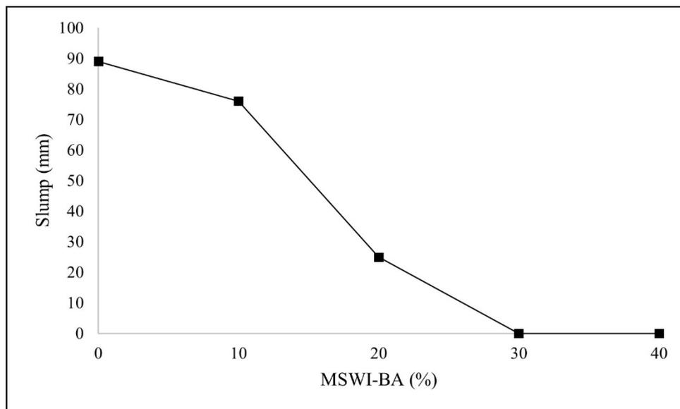
Figure 3. Slump of cement mortar containing MSWI-BA, with data from [88].
