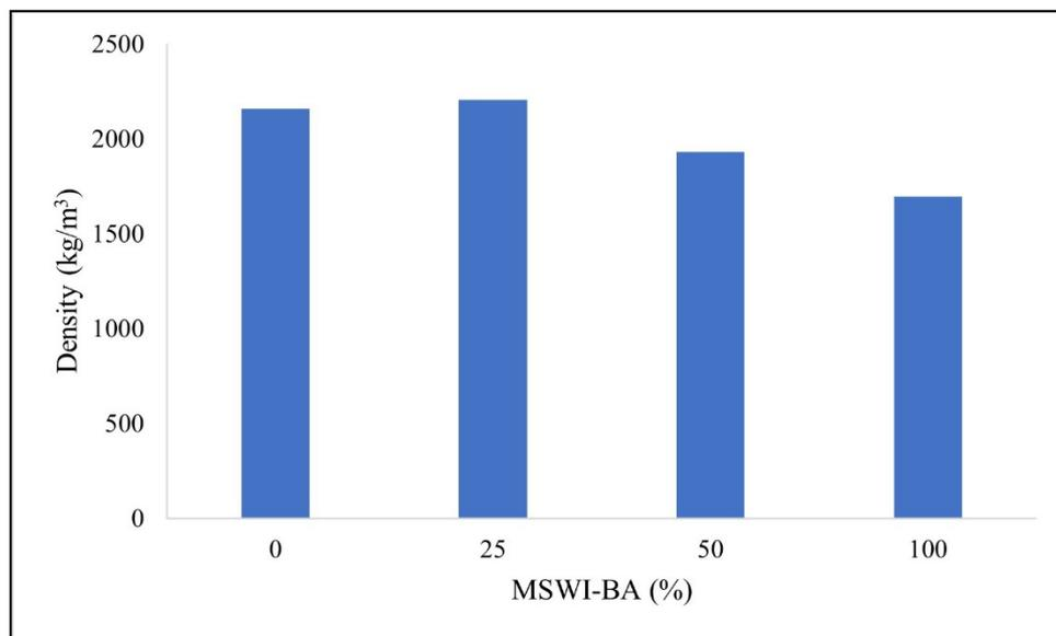
**Figure 4.** Density of the mortar containing MSWI-BA, redrawn from [46].
