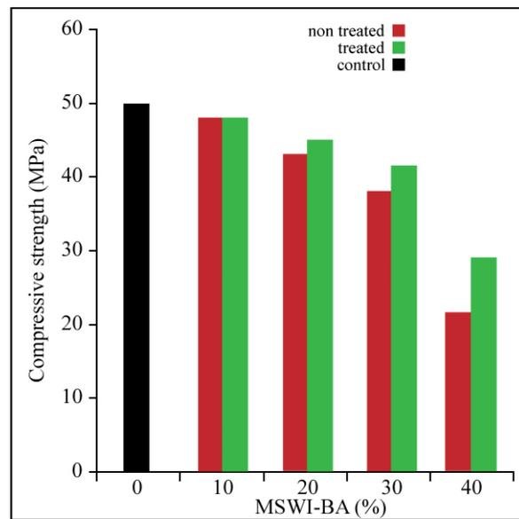
**Figure 5.** Effect of the chemical treatment of MSWI-BA on the compressive strength of concrete at 28 days, redrawn from [37].
