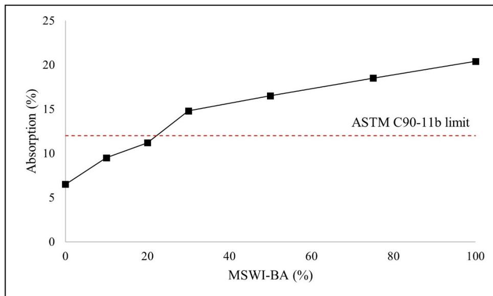
**Figure 7.** Water absorption of concrete masonry blocks, redrawn from [91].
