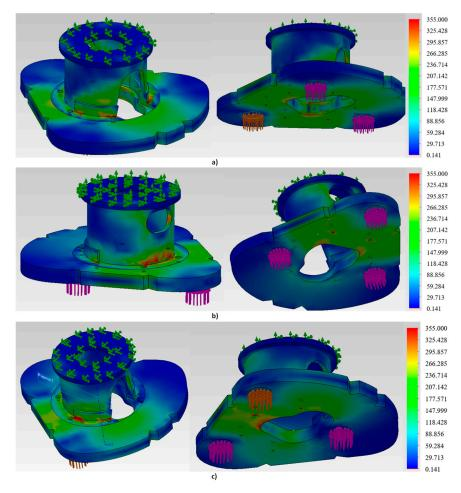
**Figure 18.** Finite Elements Model adopted to design the tripod: stress-field (N/mm<sup>2</sup>) according to the Von Mises criterion, for (a) static loading combination a, and for seismic loading combination (b)  $b_1$ , and (c)  $b_2$ .
