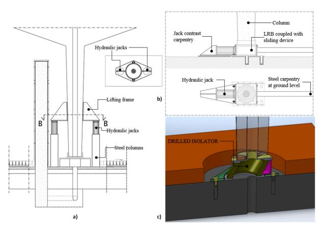
**Figure 7.** Feasibility study and first proposals of technical solutions: (a) lifting system to cut the columns, (b) thrusting system, (c) drilled Lead Rubber Bearing (LRB) isolator to house the sewage duct.
