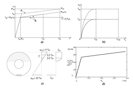
**Figure 5.** Some details of the safety evaluation: constitutive law of (a) reinforcing steel, and (b) confined concrete; (c) circular crown reinforced concrete cross-section strain and stress distribution; (d) resulting moment-curvature diagram.
