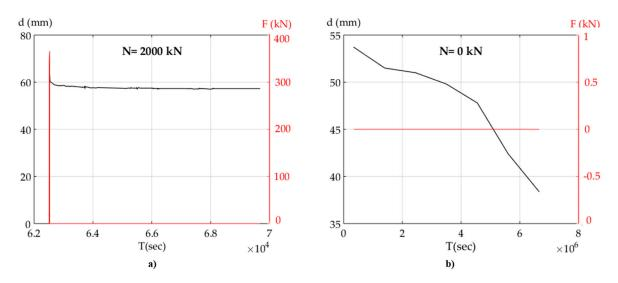
**Figure 24.** A Relaxation test [49] carried out on a real-scale LRB specimen: imposed force F(t) and displacement d(t) time histories for, (a)  $62.4 \le t \le 69.4$  ksec and constant value of applied axial load  $N_{Sd} = 2000$  kN and for, (b) 76.87 ksec  $\le t \le 6.65$  Msec and vanished axial load  $N_{Sd} = 0.0$  kN (data from [49]).
