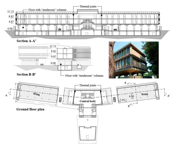
Figure 2. Plan, sections, and angular view of the building (all dimensions in m).
