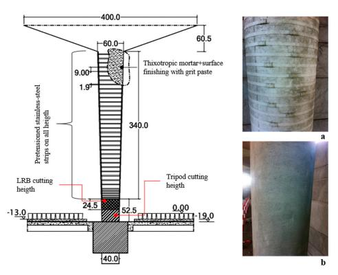
**Figure 8.** Preliminary shear strengthening of the ground floor RC columns: (a) pretensioned strips after applying a gripping layer, and (b) view of the strengthened column after applying the plaster (all dimensions in cm).
