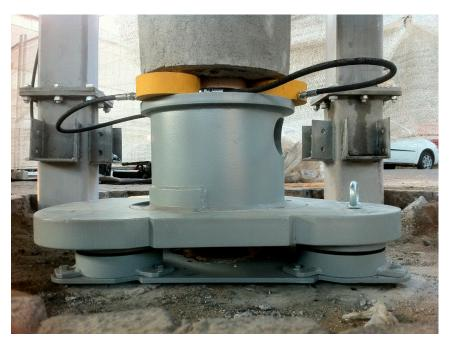
Figure 19. Picture of one of the tripods during its loading by means of three hydraulic jacks.
