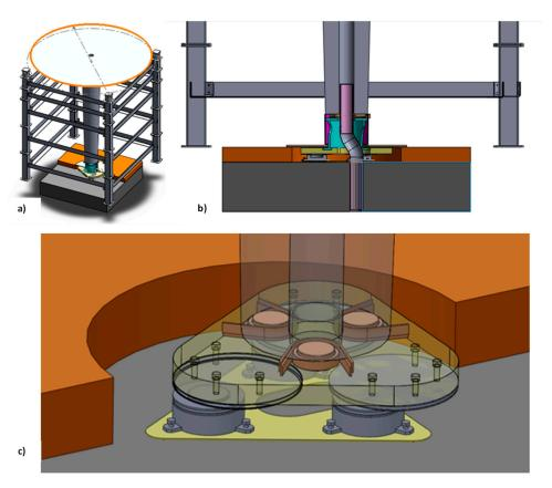
Figure 17. Technical drawings of the tripod made during their conception/design: (a) axonometric rendering of a whole mushroom-shaped column, (b) vertical cross section, and (c) close-up axonometric rendering of a tripod.
