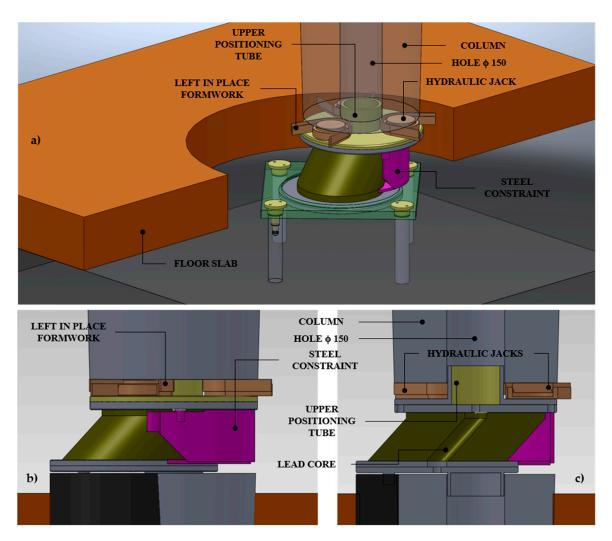
**Figure 15.** Some technical drawings (renderings) of the pre-deformed LRB isolator: (a) axonometric view; (b) lateral view; (c) vertical cross section along the diameter corresponding with the direction of translation.
