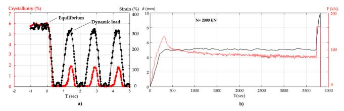
**Figure 23.** Crystallinity and Relaxation for Natural Rubbers (NRs): (a) crystallinity as a function of time under dynamic loading at a frequency of 1 Hz (data from [46]); (b) time histories of displacement (black line) and applied force (red line), for a displacement-controlled test on a LRB isolator with diameter of 45 cm (data from [49]).
