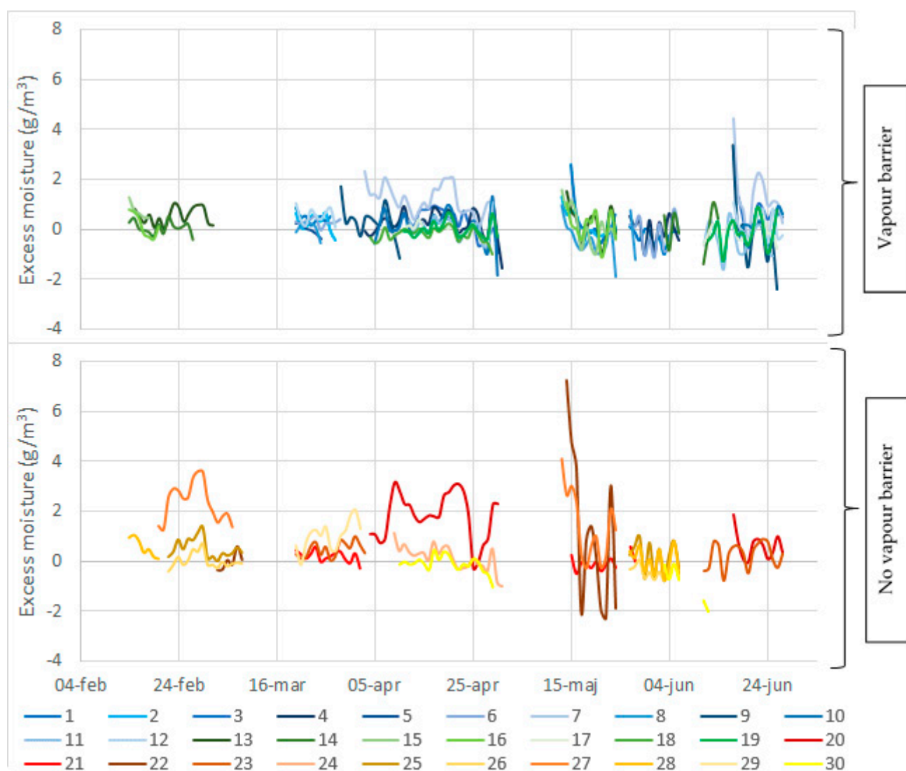
Figure 10. Daily average of excess moisture in the attics. Note that some measurements from house 22 exhibit excess moisture up to 16 g/m 3 in single measurements. Top: houses with vapour barriers (1–19), bottom: houses without vapour barriers (20–30).
