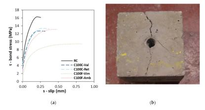
Figure 1. (a) Bond stress vs. slip curves and (b) failure mode of specimens.
