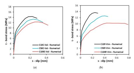
**Figure 9.** Numerical bond vs. slip curves of concrete mixes with (**a**) CRA from Valnor and (**b**) FRA from Vimajas.
