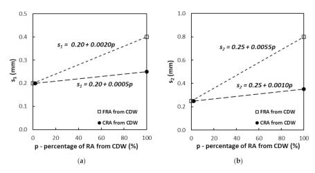
Figure 8. Variation of (a) s1 and (b) s2 with the percentage of NA replaced with RA from CDW.
