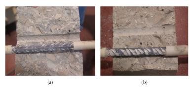
Figure 2. Mobilization of ribs in (a) RC and (b) C100F-Amb.
