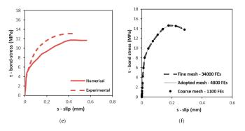
**Figure 5.** Numerical vs. experimental bond-slip curves of (**a**) RC, (**b**) C100C-Val, (**c**) C100C-Ret, (**d**) C100F-Vim, (**e**) C100F-Amb and (**f**) influence of mesh discretization on the bond-slip behavior of RC.
