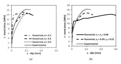
**Figure 6.** Influence of (**a**) the value of  $\alpha$  and (**b**) the adoption of  $s_1 = s_2 = 0.60$  in the numerical bond-slip curve of RC.
