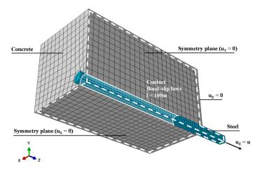
Figure 4. Geometry and mesh of the FE model developed.
