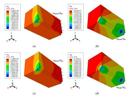
**Figure 7.** Numerical (**a**) tensile and (**b**) compressive stress fields of RC and (**c**) tensile and (**d**) compressive stress fields of C100F-Vim at the corresponding instants of maximum bond stress (stress values in MPa).
