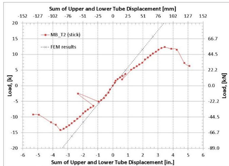
Figure 17. SAP2000 FEM with pure-rack boundary condition compared to physical test data of MB\_T2 (note that 1 in = 25.4 mm) [based on [44,51]].
