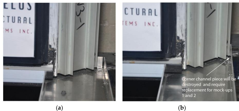
**Figure 14.** Channel of Panel 4 with representations of Panel 3 movement (a) initial position; (b) unitized sway boundary displaced position.
