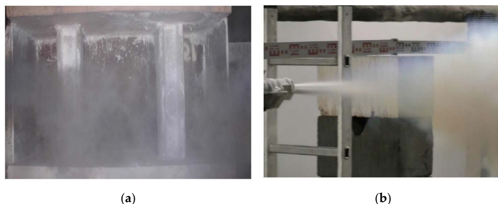
Figure 3. (a) I sections coated with Chartek after exposure to two-phase spray exposure; (b) two-phase spray generating a condition at the steel surface equivalent to immersion in a cryogenic liquid at -145^{\circ}\text{C} .
