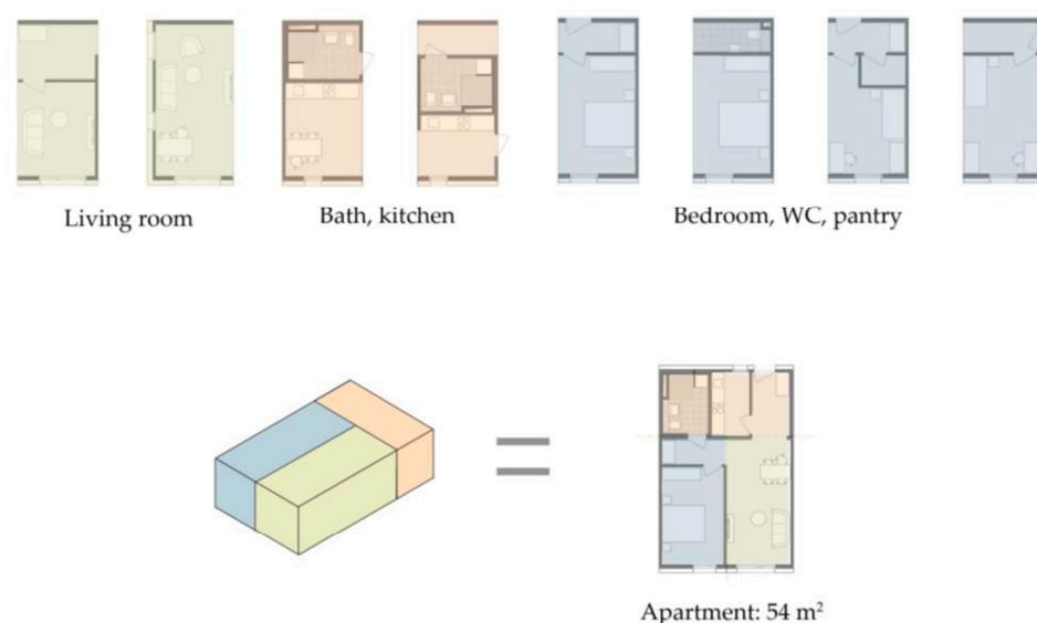
**Figure 4.** Residential unit design based on system-based modules by Firmengruppe Max Bögl/maxmodul (self-elaboration, based on data from [55]).
