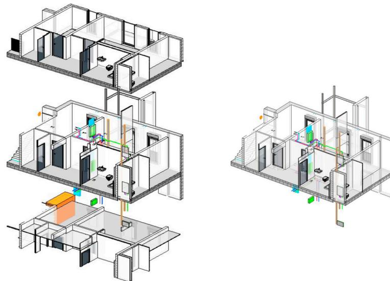
**Figure 7.** Central 3D model of a residential building consisting of prefabricated elements manufactured by GOLDBECK GmbH. Original work based on materials supplied by GOLDBECK.
