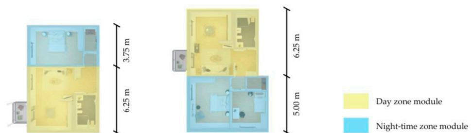
**Figure 5.** Floor plans showing a two-room and three-room units by GOLDBECK GmbH with day and night-time zones marked (self-elaboration, based on data [57]).
