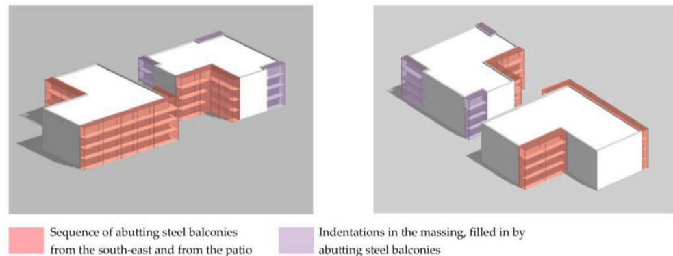
**Figure 6.** Design proposal that assumes the application of abutting, self-supported balconies by GOLDBECK GmbH. Original work based on materials supplied by GOLDBECK.
