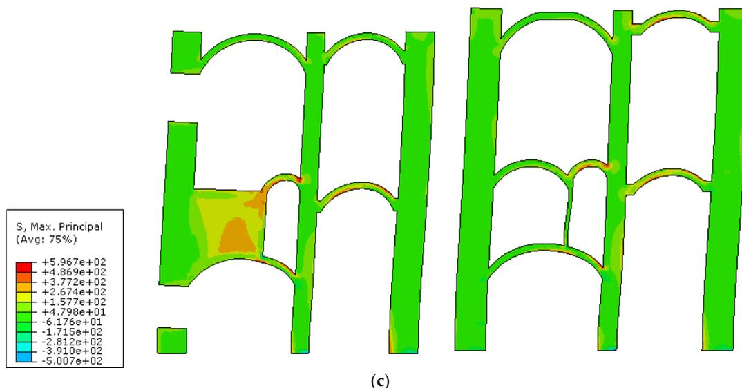
**Figure 14.** Plot extracted from the FEM. Stress gradient in relation respectively to the cross-sections A-A' and B-B' placed as in Figures 3 and 4: (a) dead weight; (b) outwards seismic action; (c) inwards seismic action. The stresses are between  $5.9 \times 10^2$  and  $-5 \times 10^2$  (kPa).
