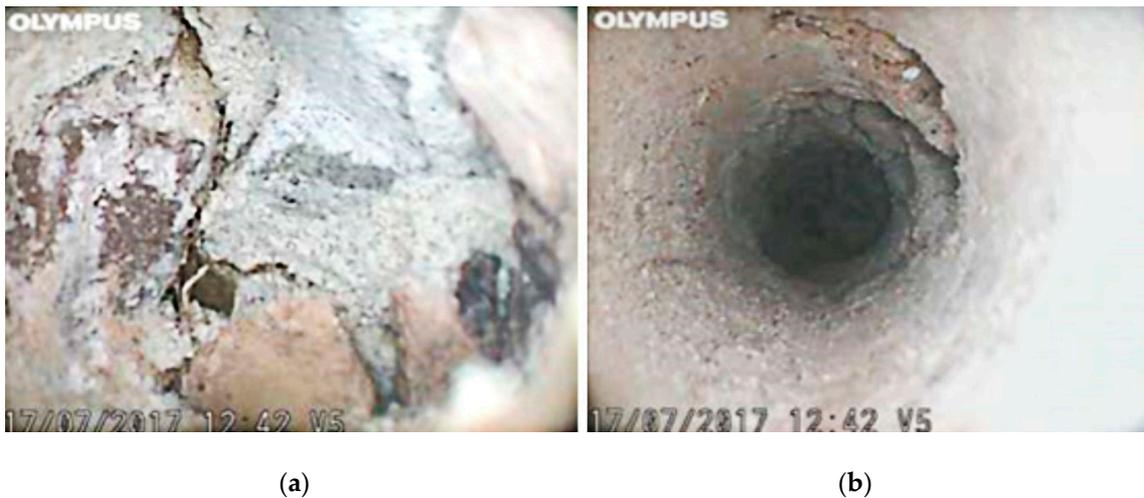
**Figure 10.** Videoendoscopy V5—from ceiling: (a) Image at 11 cm from the beginning of the hole reveals filling in unbound material; (b) Image at 5 cm from the beginning of the hole presents brick and mortar elements.
