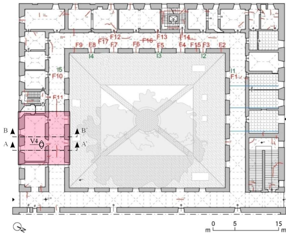
**Figure 3.** Survey of plan of the first floor completely out ground (level of the Church of Montemorcinio Nuovo;  $h = 0.0$  m): red lines—main lesions on the vaults, blue lines—steel ties installed after the 1997 earthquake. Location of the monitoring instruments: F1–F17 crack-meters, I1–I5 inclinometers, V4 videoendoscopy. The span selected for the following FEM is highlighted in red.
