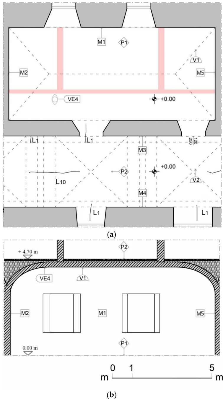
**Figure 9.** Survey of the ground floor span of Vanvitelli's Modulus: (a) The plan: in light red, the bulk of the overhead in falso walls; (b) an extract from a generic cross section, where: lesions on the structural elements (L), masonry walls (M), pavings (P), masonry vaults (V), videoendoscopies (VE).
