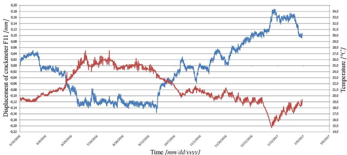
**Figure 11.** Some results of the monitoring systems (the location of the instruments is shown in Figure 3). The recordings of the crack-meter F11 are marked in red in relation to that of the thermo-hygrometer in pale blue: displacement (-) stands for crack's closure; displacement (+) coincides with an opening of the cracks.
