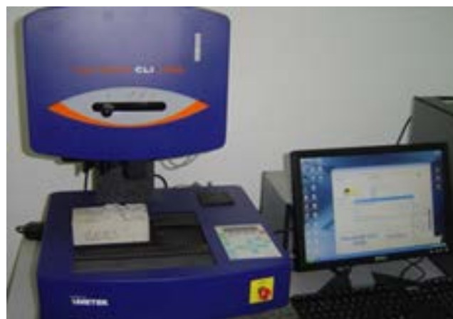
Figure 2. Talysurf CLI 1000 laser profilometer manufactured by Taylor Hobson for fast non-contact measurement of 3D surface topography.
