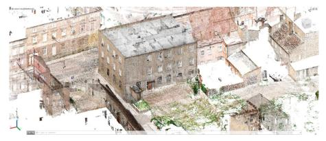
Figure 8. Outside view of the building made using TLS in Autocad 2015—axonometry.
