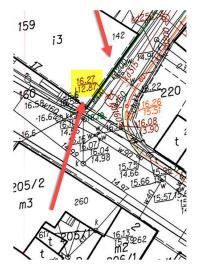
Figure 11. Ground work map—ordinate of replaced pipe near studied building.
