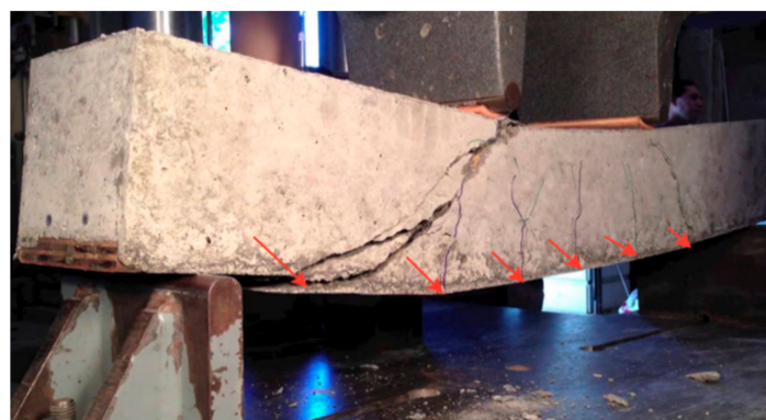
Figure 6. Destruction of a simply supported reinforced concrete beam under the action of concentrated forces.
