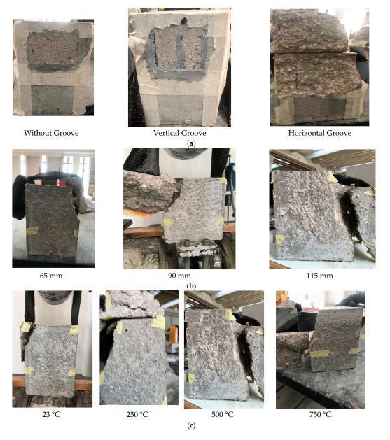
**Figure 5.** Typical mode of failure. (a) Specimens with different drilling diameters; (b) specimens with different CFRP bonded lengths; (c) specimens with different temperature degrees.
