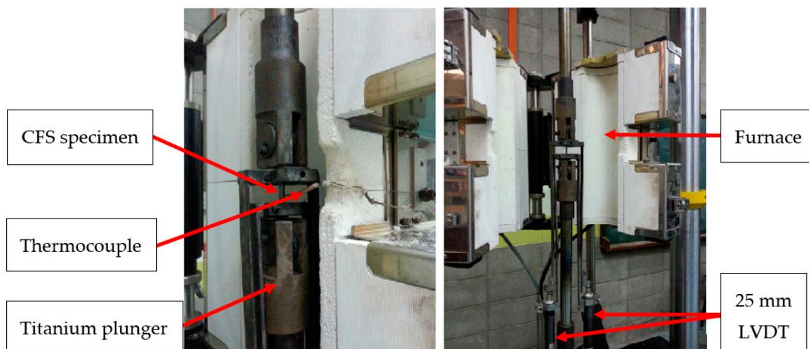
Figure 2. Testing set-up of high temperature tensile test.
