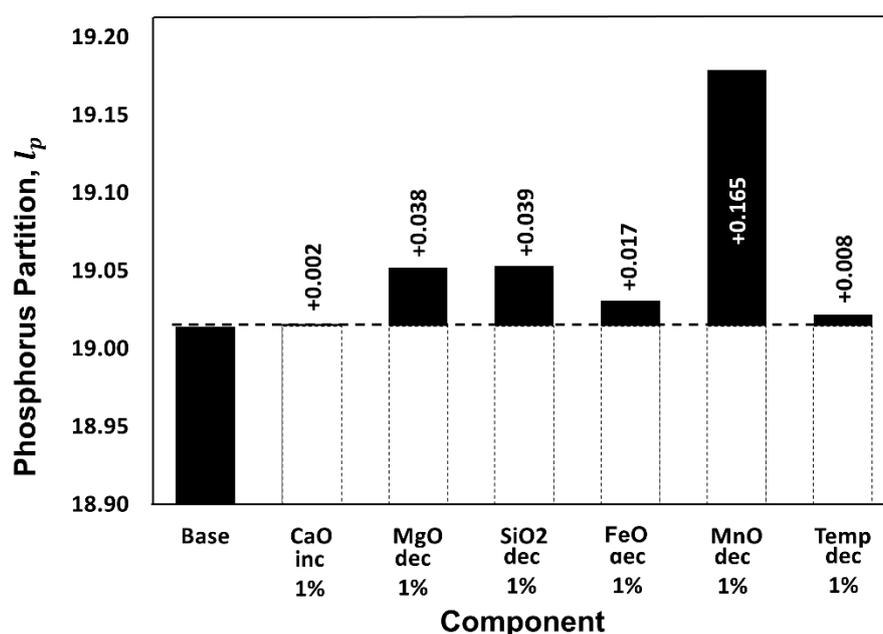
Figure 9. A waterfall analysis of the components in predicting phosphorus partition for plant II.
