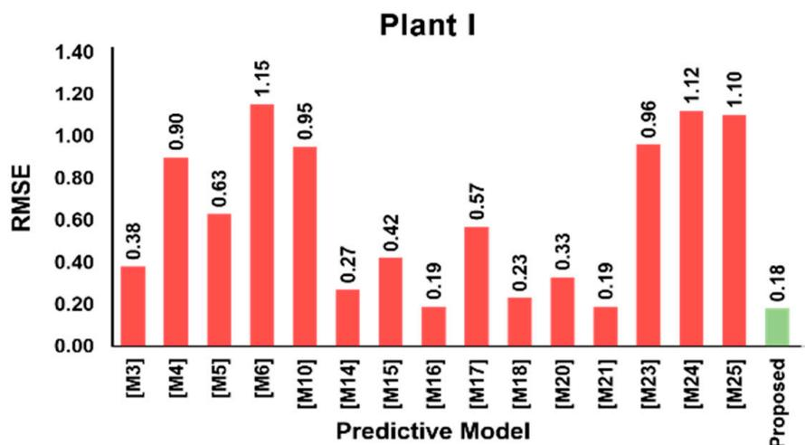
Figure 11. Comparison of root mean squared error (RMSE) values for existing and proposed models for predicting dephosphorization in steel for Plant I.
