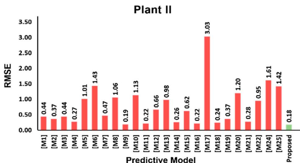
**Figure 13.** Comparison of RMSE values for existing and proposed models for predicting dephosphorization in steel for Plant II.
