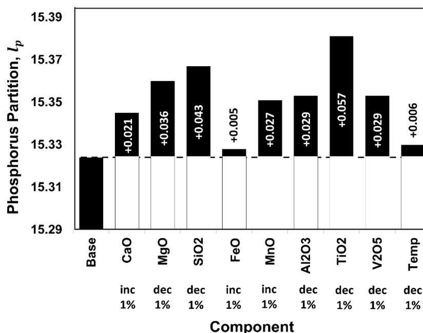
Figure 8. A waterfall analysis of the components in predicting phosphorus partition for plant I.
