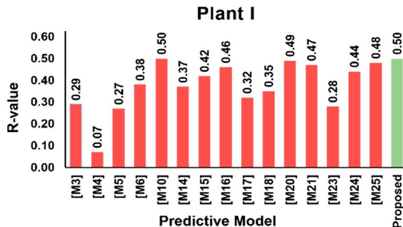
Figure 10. Comparison of R values for existing and proposed models for predicting dephosphorization in steel for Plant I.
