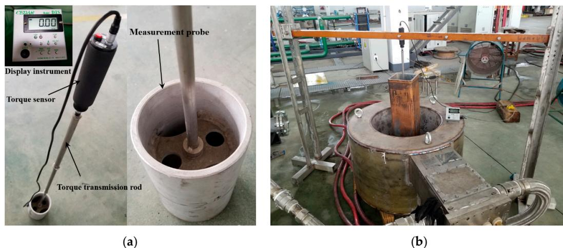
Figure 3. Structure photo of the electromagnetic torque measurement device: (a) torque meter; (b) offline test equipment.
