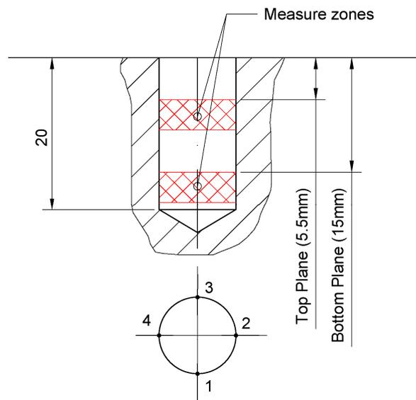
**Figure 3.** Cylindrical sections inside the holes where the measurements of roughness were taken for the evaluation of average roughness ( $Ra$ ) (striped in red) and, in each one of them, the specific zones to take the measurements are defined by the four points separated to  $90^\circ$  and marked as 1, 2, 3, and 4.
