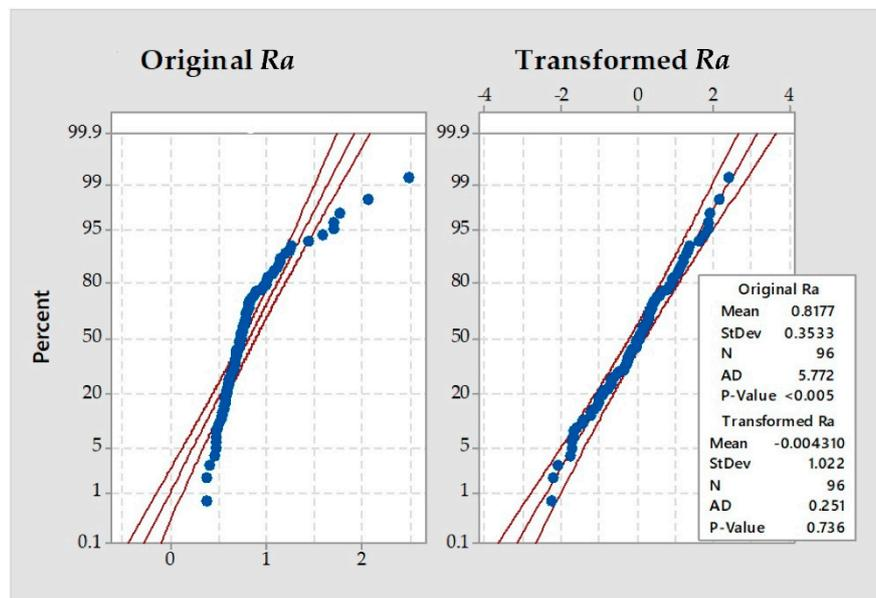
**Figure 5.** Probability plots of original non-normal data and Johnson transformed data of the  $Ra$ .
