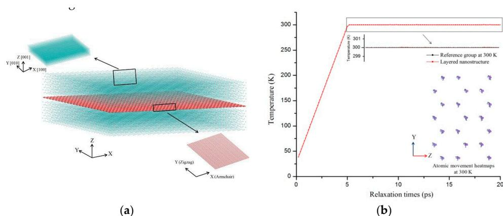
**Figure 2.** Graphene/copper layered composites. (a) Perspective side-view of graphene/copper layered composites model. Blue color represents copper atoms and red color represents carbon atoms. (b) Relaxation process of layered composites.
