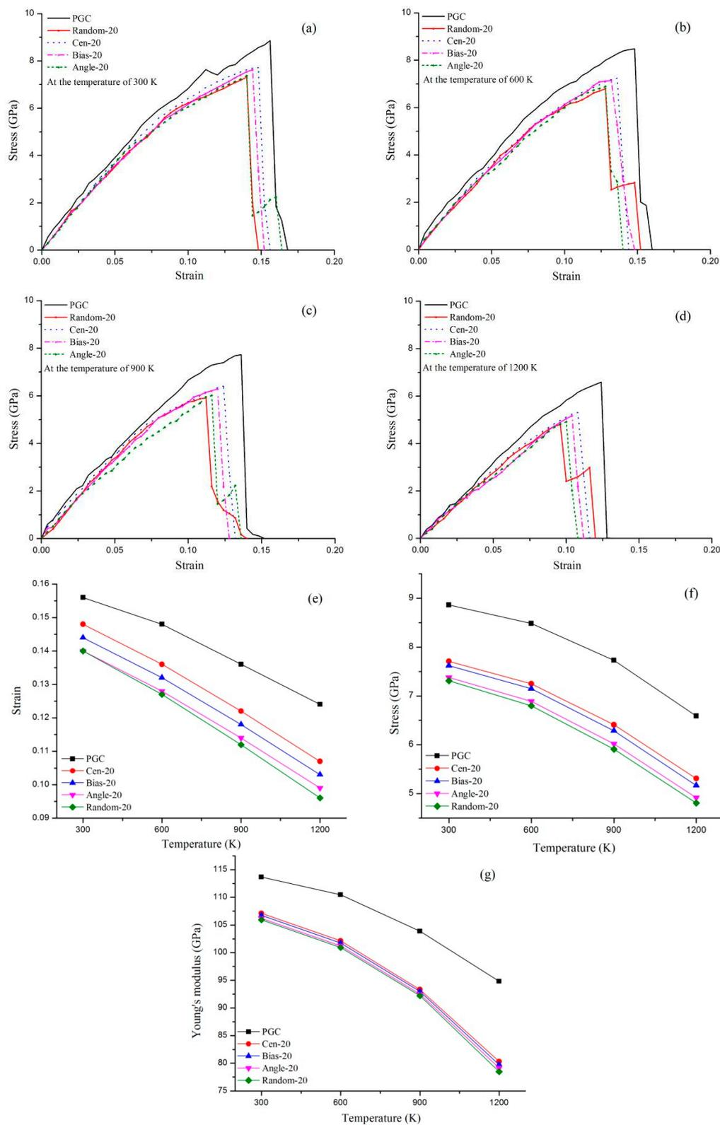
**Figure 8.** Stress-strain curve of graphene/copper layered composites with different types of defects at (a) the temperature of 300 K, at (b) the temperature of 600 K, at (c) the temperature of 900 K, and at (d) the temperature of 1200 K. (e)–(g) are mechanical values of graphene/copper layered composites with different types of defects at different temperatures.
