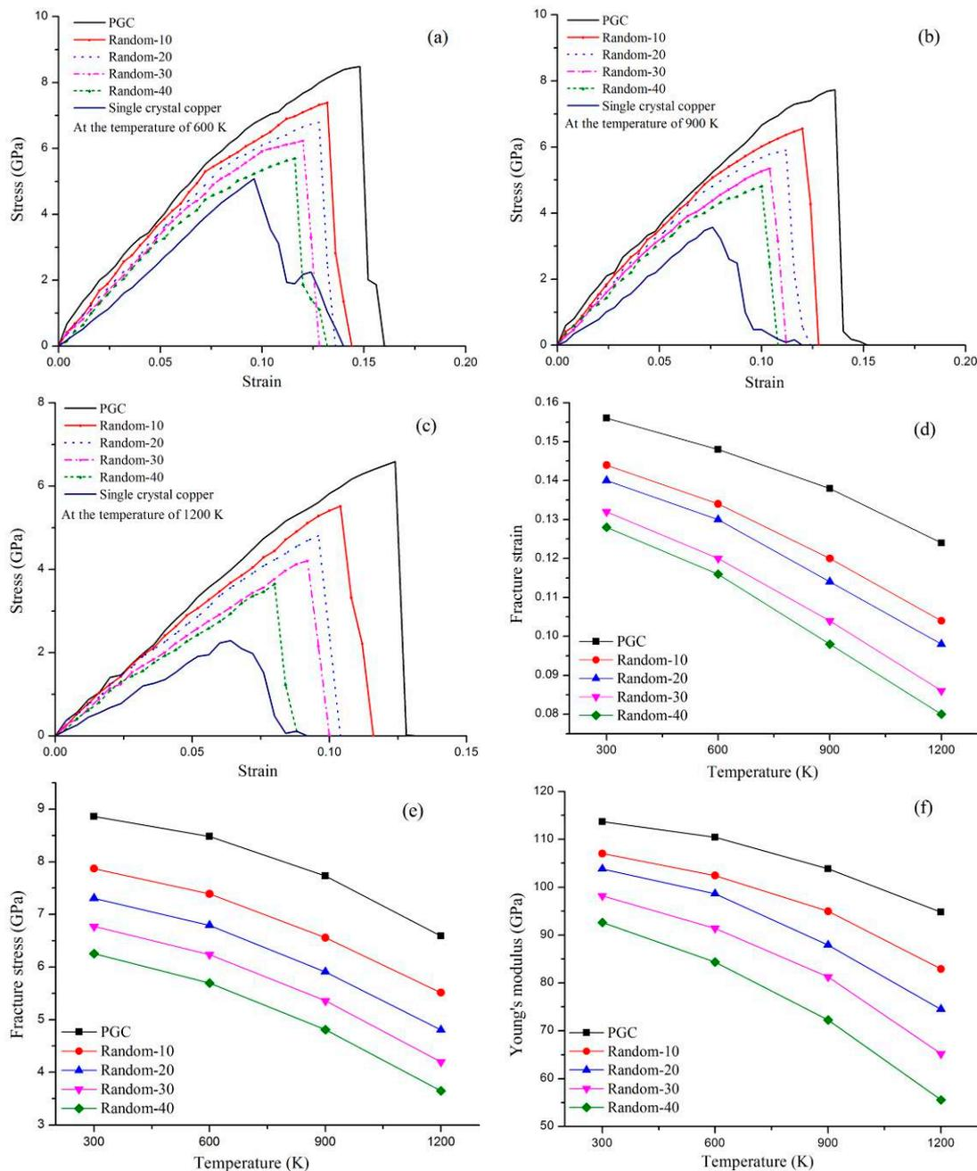
**Figure 6.** Effect of ion irradiation and temperature coupling on mechanical properties of graphene/copper layered composites in different cases. Stress-strain curve of the simulated model at (a) the temperature of 600 K, at (b) the temperature of 900 K, and at (c) the temperature of 1200 K. (d–f) Variations of fracture strain, fracture stress, and Young's modulus values of graphene/copper layered composites at different temperatures.
