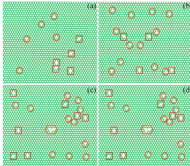
**Figure 1.** Configuration of graphene irradiated by a different number of incident carbon atoms (circular represents single vacancy (SV), square represents double vacancy (DV), and hexagon represents complex defects (CD)). (a) ion dose: 10 (SV: 5; DV: 5), (b) ion dose: 20 (SV: 12; DV: 4), (c) ion dose: 30 (SV: 11; DV: 7; CD: 1), and (d) ion dose: 40 (SV: 19; DV: 10; CD: 2).
