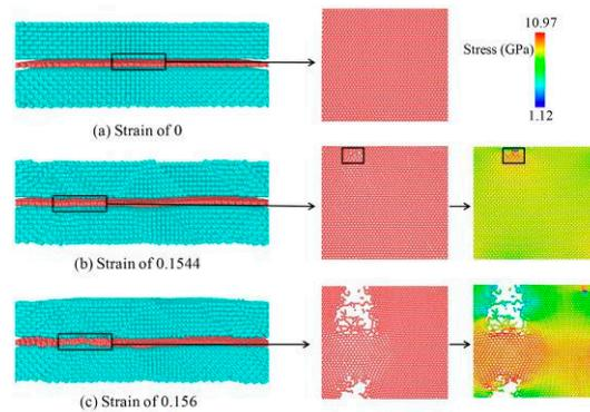
**Figure 4.** Fracture process and stress distribution of PGC under uniaxial tensile loading at the temperature of 300 K. (a)  $\varepsilon = 0$  before the load is applied. (b)  $\varepsilon = 0.1544$  before reaching the stress limit. (c)  $\varepsilon = 0.156$  after Fracture Failure.
