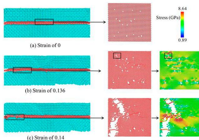
**Figure 5.** Fracture process and stress distribution of Random-20 under uniaxial tensile loading at the temperature of 300 K. (a)  $\varepsilon = 0$  before the load is applied. (b)  $\varepsilon = 0.136$  before reaching the stress limit. (c)  $\varepsilon = 0.14$  after fracture failure.
