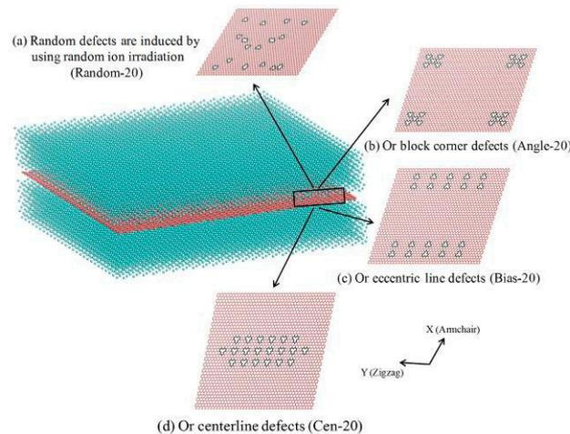
**Figure 7.** Local side view of graphene with various defects inserted into copper. (a) Random defects are induced by 20 randomly ions irradiation. (b) Block corner, (c) eccentric line, and (d) centerline defects are created in graphene by using 20 directional ions irradiation.
