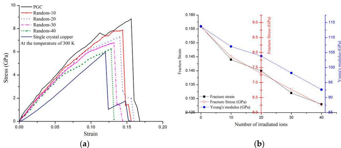
**Figure 3.** Mechanical properties of graphene/copper layered composites. (a) Stress-strain curves and (b) mechanical values of graphene/copper layered composites and single crystal copper (Random -10, -20, -30, and -40 represent graphene/copper layered composites with various defects, which are created by using 10, 20, 30, and 40 doses of atoms, respectively).
