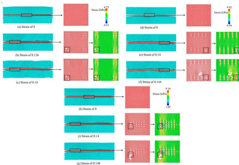
**Figure 9.** Fracture process and stress distribution of graphene/copper layered composites with (a–c) centerline, with (b–f) eccentric line, and with (h–g) block corner defects at the temperature of 300 K. (Before the load is applied, before reaching the stress limit, and after fracture failure).
