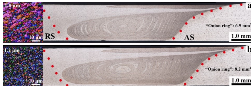
Figure 6. The cross-section of the FSW joints produced by (a) the 0.4 mm pin-eccentric stir tool, joint P0.4, and (b) the 0.8 mm pin-eccentric stir tool, joint P0.8.
