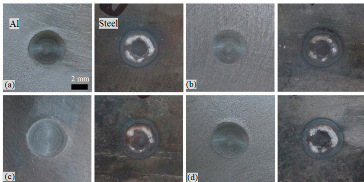
Figure 2. Photographs of the welded spots at different welding parameters of (a) 8.5 kA–300 ms, (b) 9.5 kA–200 ms, (c) 9.5 kA–300 ms with a coarse base material and (d) 9.5 kA–300 ms with a fine base material.
