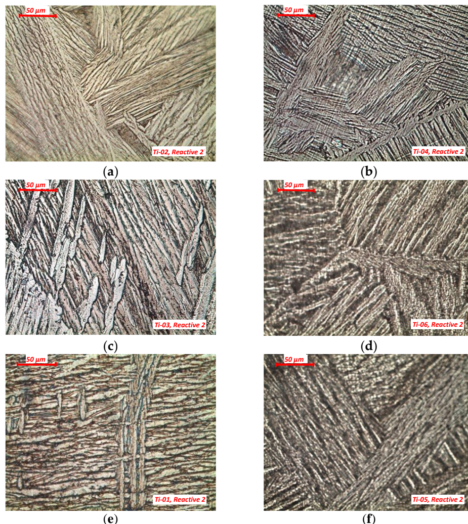
Figure 4. Optical micrographs (400 \times magnification) of the titanium ingots produced at different melting powers for different lengths of time: (a) P_b = 2.5 kW, \tau = 25 min; (b) P_b = 2.5 kW, \tau = 40 min; (c) P_b = 3.5 kW, \tau = 25 min; (d) P_b = 3.5 kW, \tau = 40 min; (e) P_b = 5.5 kW, \tau = 15 min; and (f) P_b = 5.5 kW, \tau = 40 min.
