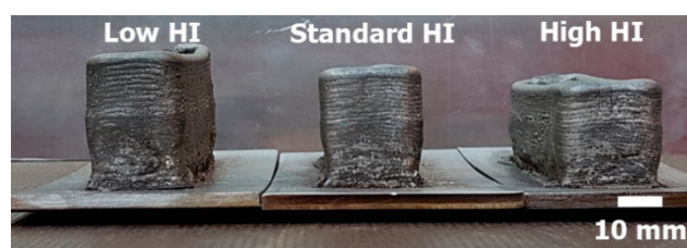
Figure 5. SS316L to Ni625 structures manufactured by 3DPMD.
