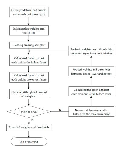
Figure 2. The improved BP algorithm flow.
