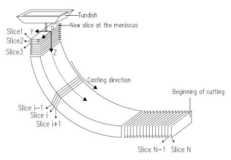
**Figure 1.** Schematic of space-time dispersion of the internal crack generation index of the slice unit in the slab casting process.
