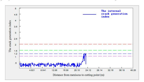
Figure 4. The internal crack generation index distribution at the beginning stage of casting.
