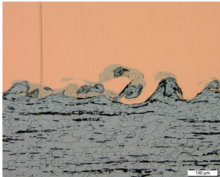
Figure 16. Weld interface at the middle of the weld.
