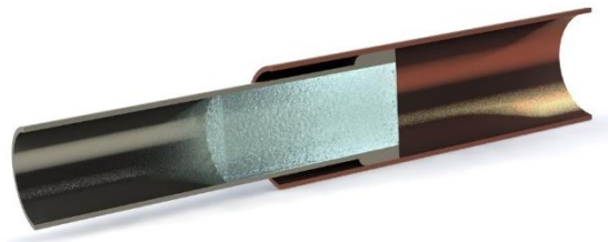
Figure 8. Joint configurations with an internal support of ice.
