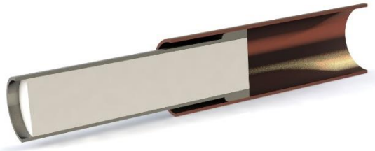
Figure 9. Joint configurations with an internal support of plaster.
