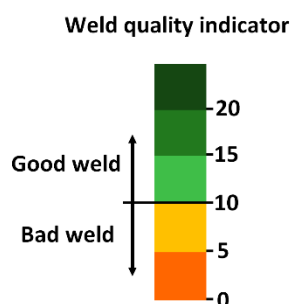
Figure 5. WQI colour scale bar to classify the weld quality, with a threshold value of 10.
