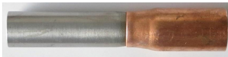
Figure 4. Example of a tubular connection realised with electromagnetic pulse welding (copper tube outer diameter: 22.22 mm).
