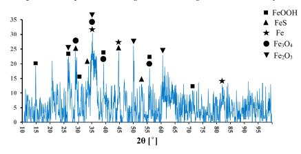
Figure 8. An X-ray diffraction analysis of the surface of the pipe.
