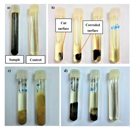
**Figure 11.** SRB growth monitoring in specific media after 20 days. Control: The specific medium without inoculation. (a) Surface scratch from corrosion tube, (b) the corrosion tube cuts (c) the soil samples of corrosion area after five days, and (d) after 20 days.
