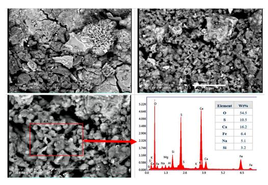
Figure 7. Examples of SEM images of biofilms together with EDS analysis.
