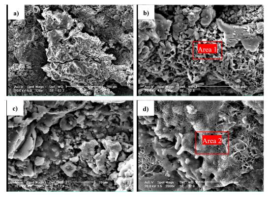
**Figure 9.** Different morphologies of the corrosion products at the inner surface: (**a**) and (**b**) scale-like layer intermingled with some globular  $\alpha$ -FeOOH particles, (**c**) plate-like micaceous crystalline features, and (**d**) honeycomb-like structures.
