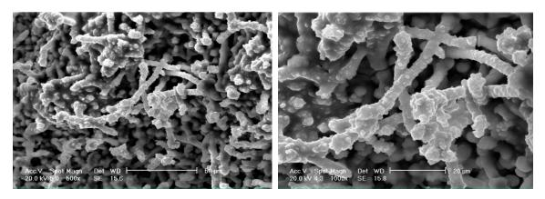
**Figure 14.** Corrosion products development after reactivation of SRB due to inoculation of the corroded tube cuts in the SRB-specific media (Images are from similar features with different magnifications).
