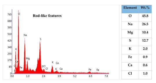
Figure 13. An EDS analysis of area shown in Figure 12 (x-axis: Energy (KeV), y-axis: a.u.).
