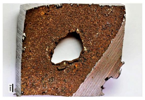
Figure 3. An inner surface of the failed elbows.
