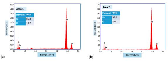
Figure 10. EDS analyses of (a) area 1 and (b) area 2, shown in Figure 9.
