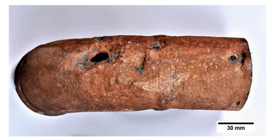
Figure 2. An example of the failed elbows.
