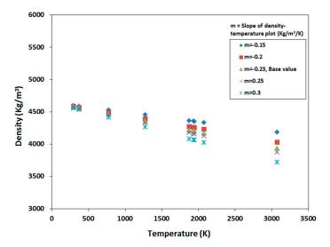
Figure 8. Density vs temperature plot with varying slopes.
