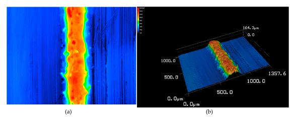
**Figure 6.** (a) Two-dimensional and (b) three-dimensional confocal microscopy images of single beads Ti-64 samples produced at laser power of 400 W at scanning speed of 200 mm/s.
