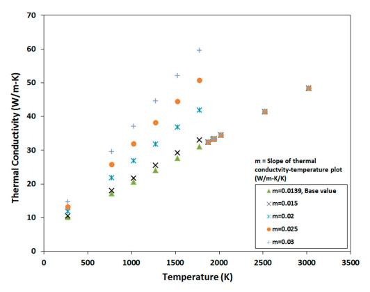
Figure 11. Slope of thermal conductivity data before melting point is varied.
