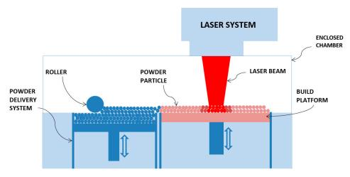
Figure 1. Schematic of Selective Laser Melting (SLM) system.
