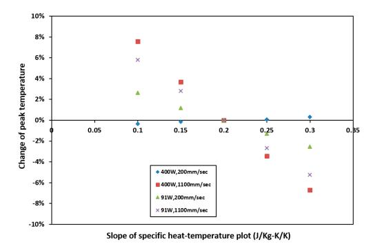
**Figure 14.** Sensitivity of peak temperature to specific heat. Percentage change of peak temperature with respect to that calculated with base specific heat at different process parameters.
