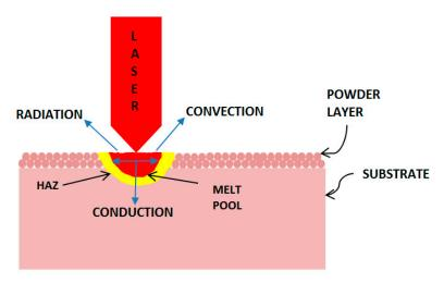
Figure 2. Schematic of energy transport mechanisms in the laser processed zone.
