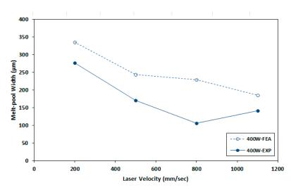
Figure 7. Melt-pool width of Ti-64 beads at 400 W laser power and 200-1100 mm/s sweeping speed.
