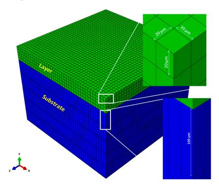
**Figure 3.** Single layer of Ti-64 on top of a substrate. In this particular case, the substrate material is also Ti-64. Element sizes in layer and substrate are shown by zooming associated elements.
