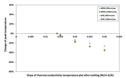
**Figure 17.** Sensitivity of peak temperature to thermal conductivity. Change of peak temperature with respect to that calculated with base thermal conductivity at varying process parameters. Slope of thermal conductivity–temperature plot *after* the melting point is varied only.
