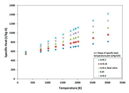
Figure 9. Sets of specific heat data by varying its slope from the base slope of 0.2 J/kg-K/K.
