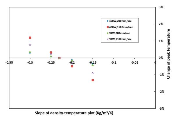
**Figure 13.** Sensitivity of peak temperature to density. Percentage change of peak temperature with respect to that calculated with base density at different process parameters.
