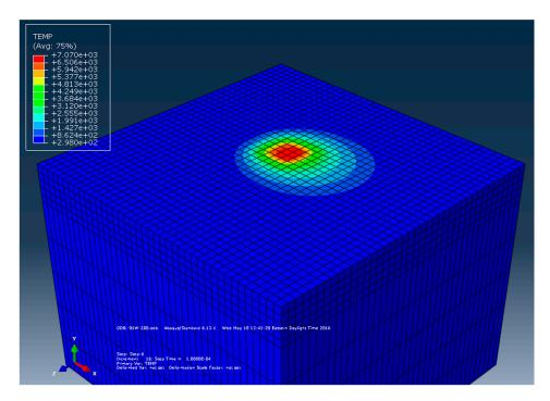
Figure 4. Surface temperature distribution at a laser power of 91 W with scanning speed, 200 mm/s.
