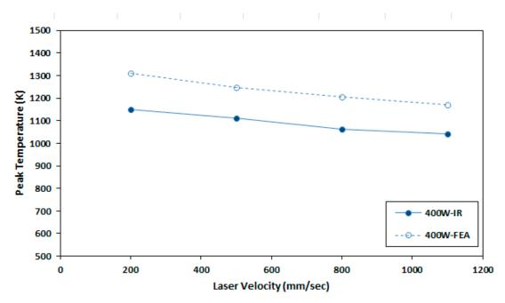
**Figure 5.** Comparison of maximum FEA temperature that is averaged over a camera pixel and IR data of Ti-64 sample at 400 W and 200 to 1100 mm/s.
