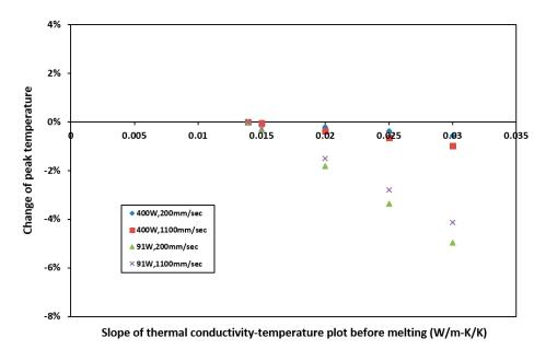
**Figure 16.** Sensitivity of peak temperature to thermal conductivity. Change of peak temperature with respect to that calculated with base thermal conductivity at varying process parameters. Slope of thermal conductivity–temperature plot *before* the melting point is varied only.
