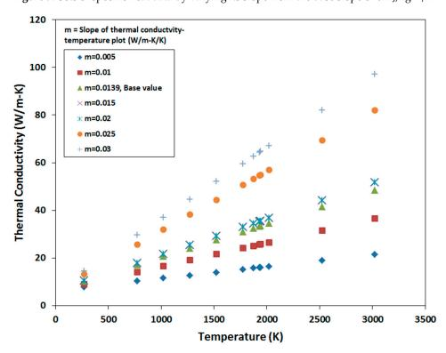
**Figure 10.** Seven sets of thermal conductivity data generated by varying the base slope (shown in Equation (7)) between 0.005 and 0.03 W/m-K/K.
