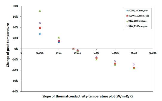
**Figure 15.** Sensitivity of peak temperature to thermal conductivity. Percentage change of peak temperature with respect to that calculated with base thermal conductivity at different process parameters.
