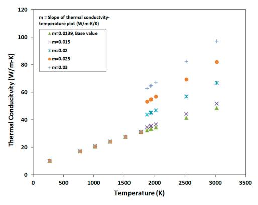
Figure 12. Slope of thermal conductivity data after the melting point is varied.
