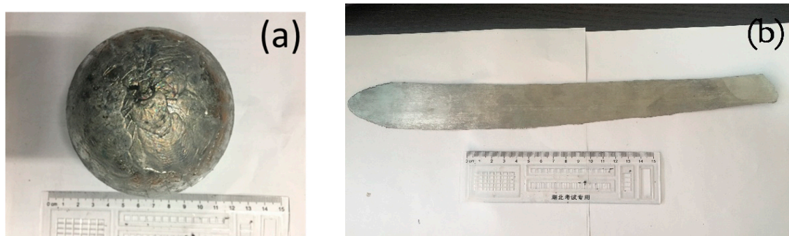
Figure 6. The macroscopic appearance: (a) (\text{Fe}_{0.3}\text{Co}_{0.5}\text{Ni}_{0.2})_{95}(\text{Al}_{1/3}\text{Si}_{2/3})_5 alloy ingot prepared by maglev melting, (b) cold-rolled sheet.
