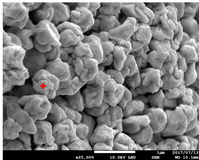
**Figure S3.** FE/SEM image of gold particles precipitated from solution by reductive precipitation with L-AA
