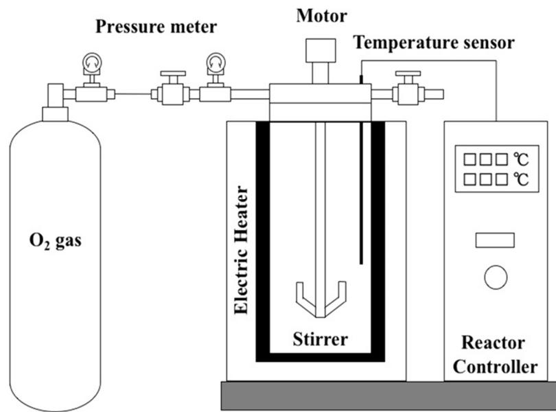
**Figure S1.** A schematic diagram of an autoclave used in this study.
