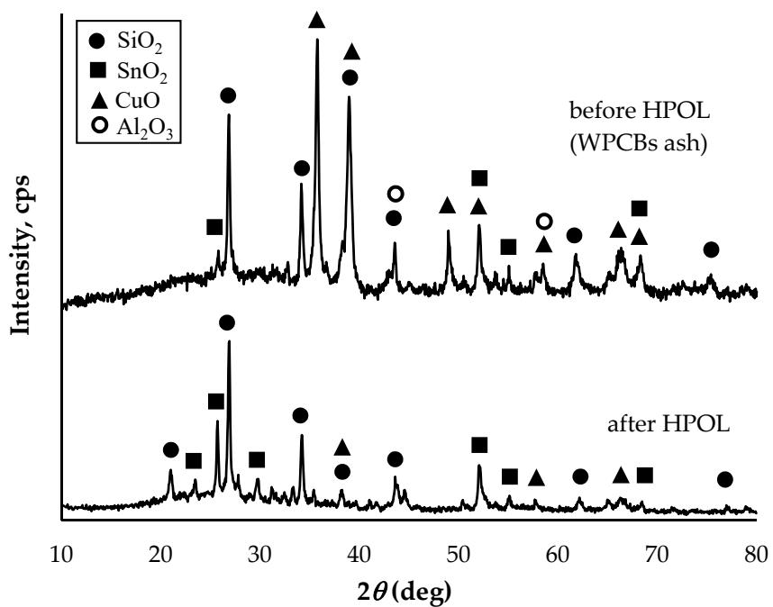
**Figure 2.** A comparison of the XRD pattern of the leach residue of HPOL with WPCBs ash sample
