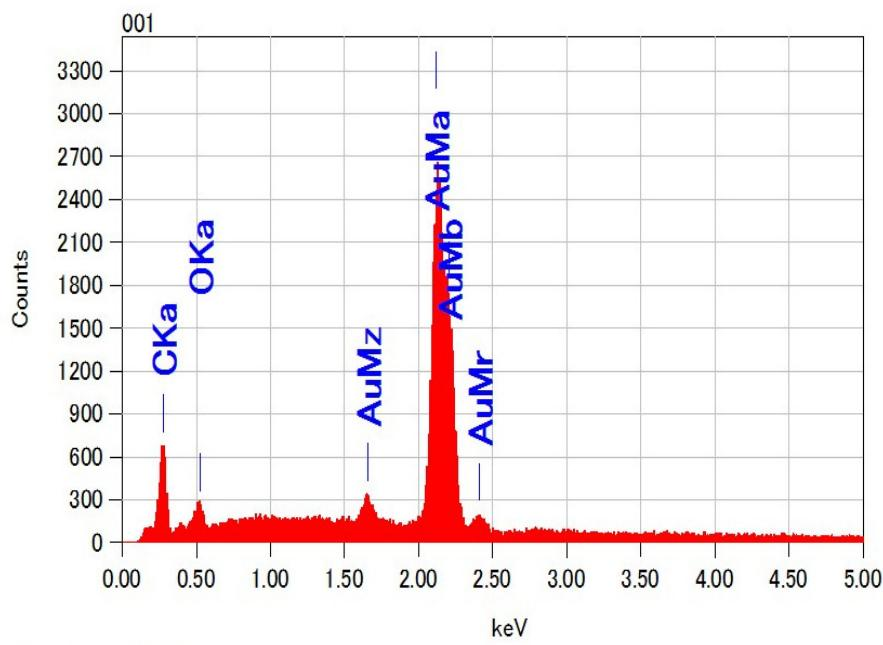
**Figure S4.** EDS spectra of gold particles precipitated from the solution by reductive precipitation with L-AA
