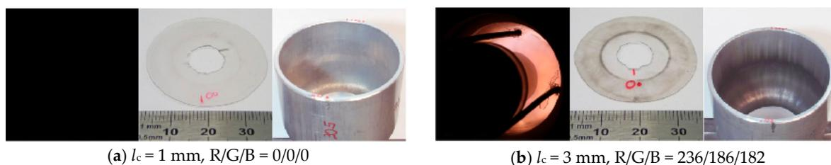
**Figure 13.** Long time exposures of the process glare, first plastic disc and flyer tube after MPW experiments at the Bmax setup ( $p = 0.1 \text{ mbar}$ ,  $\alpha = 0^\circ$ ,  $g = 1.5 \text{ mm}$ ,  $E = 4.5 \text{ kJ}$ ,  $I_{\text{max}} = 365 \text{ kA}$ ,  $\varnothing \text{ coil} = 41 \text{ mm}$ ,  $w_c = 10 \text{ mm}$ ,  $l_w = 6 \text{ mm}$ ): (a)  $l_c = 1 \text{ mm}$  (b)  $l_c = 3 \text{ mm}$ .
