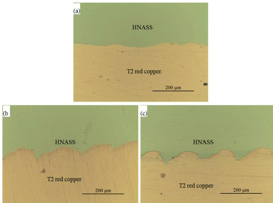
**Figure 5.** Morphologies of the joint surface for different explosive ratios. (a)  $R=0.9$ ; (b)  $R=1.1$ ; (c)  $R=1.6$ .
