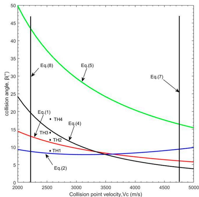
**Figure 2.** The explosive welding weldability window for the red copper and HNASS calculated using Equations (1)–(8).
