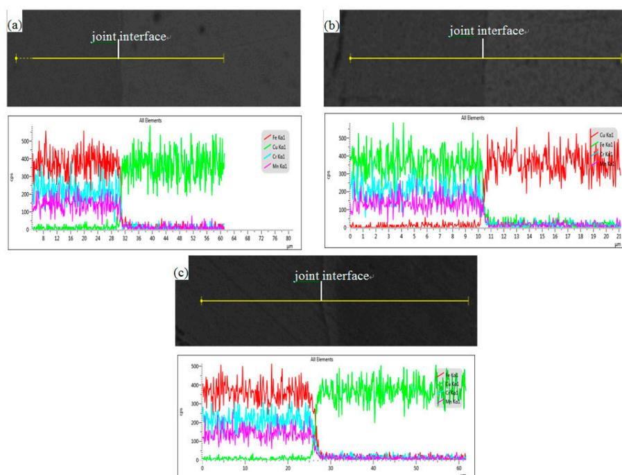
**Figure 7.** Element line scanning near the joint surface under different explosive welding conditions. (a)  $R = 0.9$ ; (b)  $R = 1.1$ ; (c)  $R = 1.6$ .
