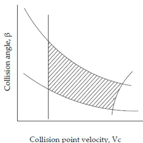
Figure 1. Weldability window for explosive welding.
