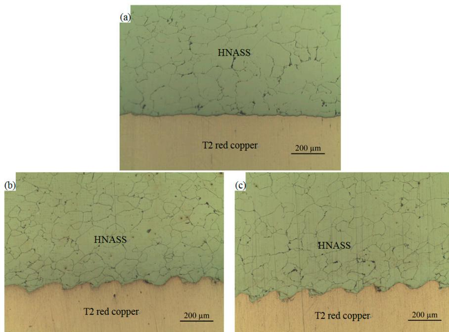
**Figure 6.** Grains of the parent plate near the joint interface for different explosive ratios. (a)  $R = 0.9$ ; (b)  $R = 1.1$ ; (c)  $R = 1.6$ .
