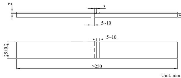
**Figure 4.** Dimensions of the tensile specimen.
