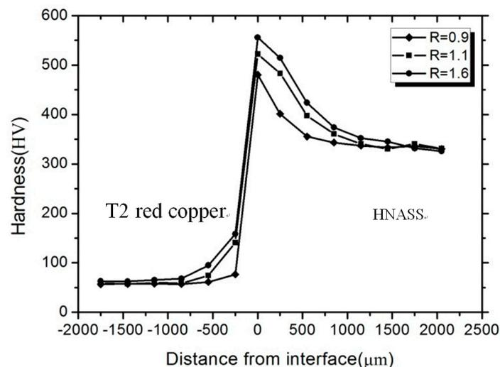
**Figure 8.** Microhardness values of T2 red copper/HNASS under different explosive welding parameter.
