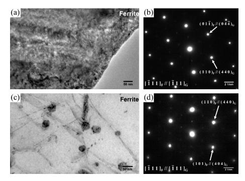
**Figure 3.** TEM results of Z3CN20.09M. (**a**) Aged at 475 °C for 2000 h and (**c**) aged at 475 °C for 2000 h then annealed at 550 °C for 3 h. (**b**,**d**) are the corresponding electron diffraction (ED) pattern of (**a**,**c**), respectively.
