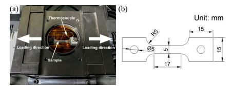
**Figure 2.** (a) The in situ tensile testing stage of VL2000DX-SVF15FTC high temperature confocal scanning violet laser microscope and (b) the dimensions of the specimen.
