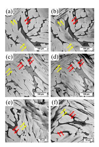
**Figure 7.** Effects of ferrite shapes on blocking the slip bands in Z3CN20.09M CDSS. Figure (**a**,**b**,**e**,**f**) were the microstructure snapshots during the in situ tensile test using the samples under the "aged 2000 h, 320 °C" condition. Figure (**c**,**d**) were the microstructures from the sample with the "annealed 3 h, 320 °C" condition. The tensile axis is along the horizontal direction in all the figures.  $\gamma$  denotes the austenite phase, and  $\delta$  is the ferrite phase.
