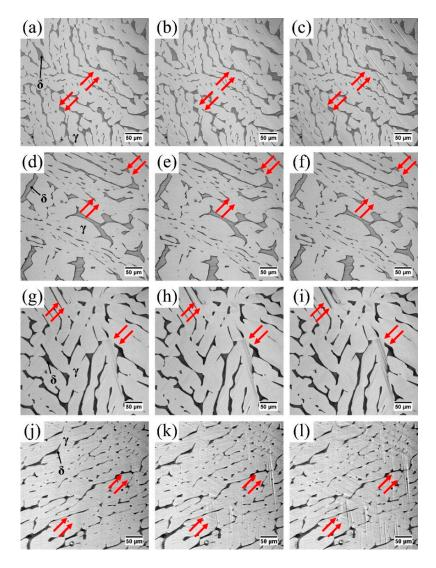
**Figure 5.** The primary stage of the plastic deformation of Z3CN20.09M CDSS. Figure (**a**–**c**) were the "as received, 20 °C" condition. Figure (**d**–**f**) were the "as received, 320 °C" condition. Figure (**g**–**i**) were the "aged 2000 h, 320 °C" condition. Figure (**j**–**l**) were the "annealed 3 h, 320 °C" condition. The tensile axis is along the horizontal direction in all the figures.  $\gamma$  denotes austenite phase, and  $\delta$  is the ferrite phase.
