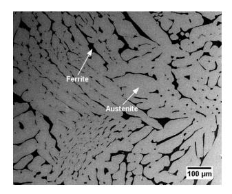
Figure 1. Typical microstructure of the Z3CN20.09M cast duplex stainless steel.
