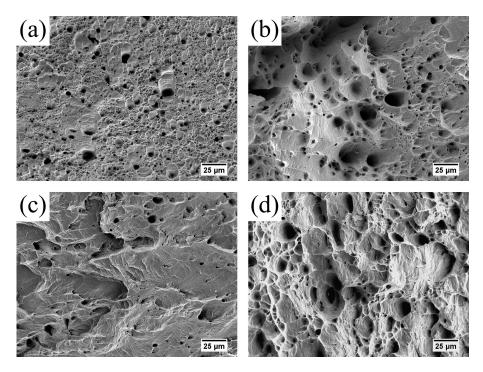
**Figure 11.** Fractographic image of Z3CN20.09M CDSS with different tensile conditions. (**a**) The "as received, 20 °C" condition; (**b**) the "as received, 320 °C" condition; (**c**) the "aged 2000 h, 320 °C" condition; (**d**) the "annealed 3 h, 320 °C" condition. Figures are imaged by SEM after tensile tests.
