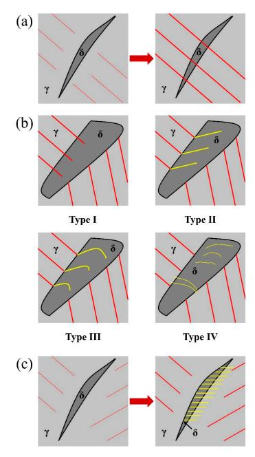
**Figure 8.** The slip deformation mechanisms of the Z3CN20.09M. (**a**) Narrow ferrite grains; (**b**) thick ferrite grains and (**c**) a certain kind of slip deformation that only happened in the thermally aged steel.
