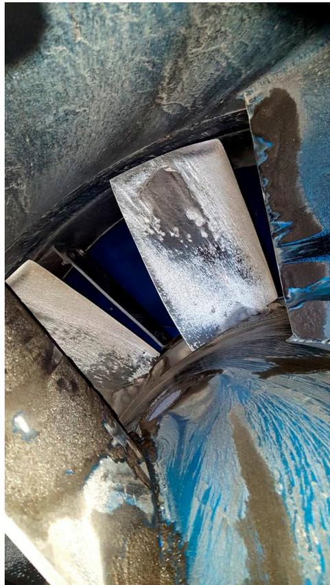
Figure 1. Mine fan subjected to erosive wear.
