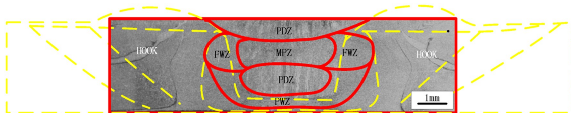
Figure 6. The macrostructure of the joint with filled keyhole.
