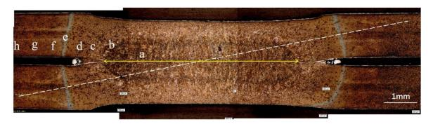
**Figure 5.** Low-magnification optical microstructure of a whole spot welding joint obtained at AC-6, with a peak current of 12 kA, frequency of 110 Hz, and welding time of 35 cycles.
