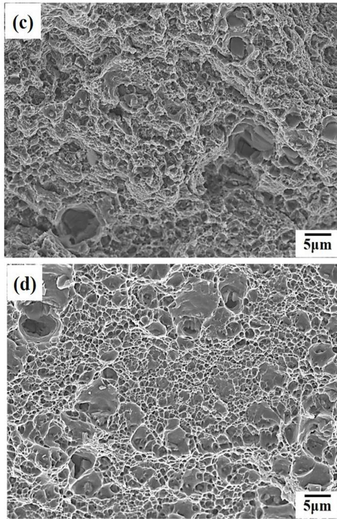
**Figure 5.** Microstructures of tensile fractures for 7075 aluminum alloy after FSP and various heat treatments: (a) BM-O specimen, (b) BM-W specimen, (c) 440-NA specimen, (d) 440-W specimen.
