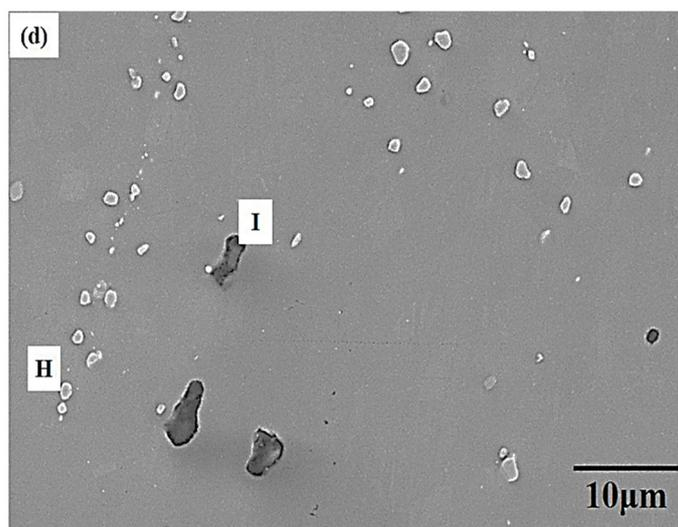
**Figure 9.** The morphology and the distribution of the 7075 aluminum alloys after FSP and various heat treatments: (a) BM-O specimen, (b) BM-W specimen (c) 440-NA specimen, (d) 440-W specimen.
