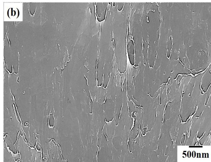
**Figure 6.** SEM images with high magnification of fractures of 440 specimens after various heat treatments (a) 440-NA specimen, (b) 440-W specimen.
