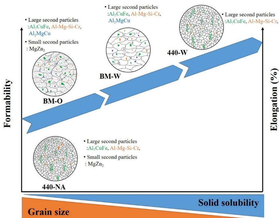
**Figure 10.** A schematic diagram of the relationships among formability, elongation, and microstructure for 7075 aluminum alloys after FSP and various heat treatments.
