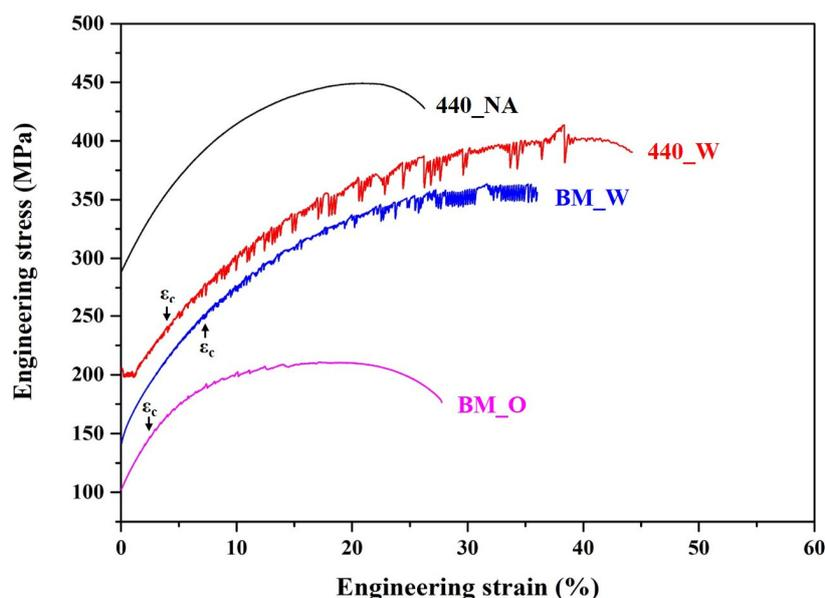
**Figure 3.** Stress–strain flow curves of 7075 aluminum alloy after FSP and various heat treatments.
