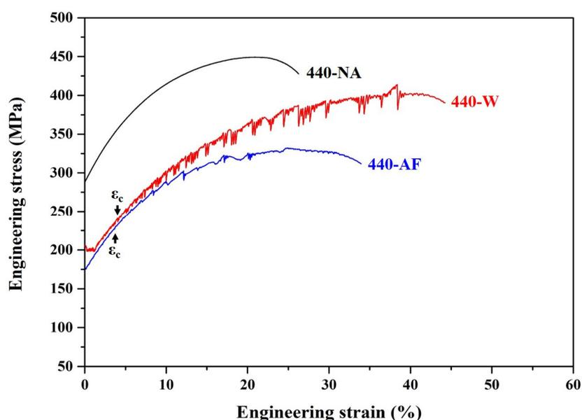
**Figure 4.** Stress–strain flow curve of FSPed specimens with different solid solubility.
