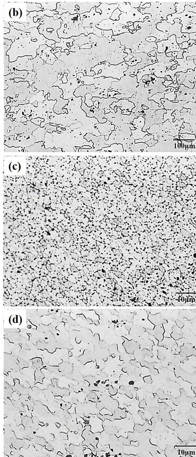
**Figure 8.** The microstructure of 7075 aluminum alloys after FSP and various heat treatments: (a) BM-O specimen, (b) BM-W specimen (c) 440-NA specimen, (d) 440-W specimen.
