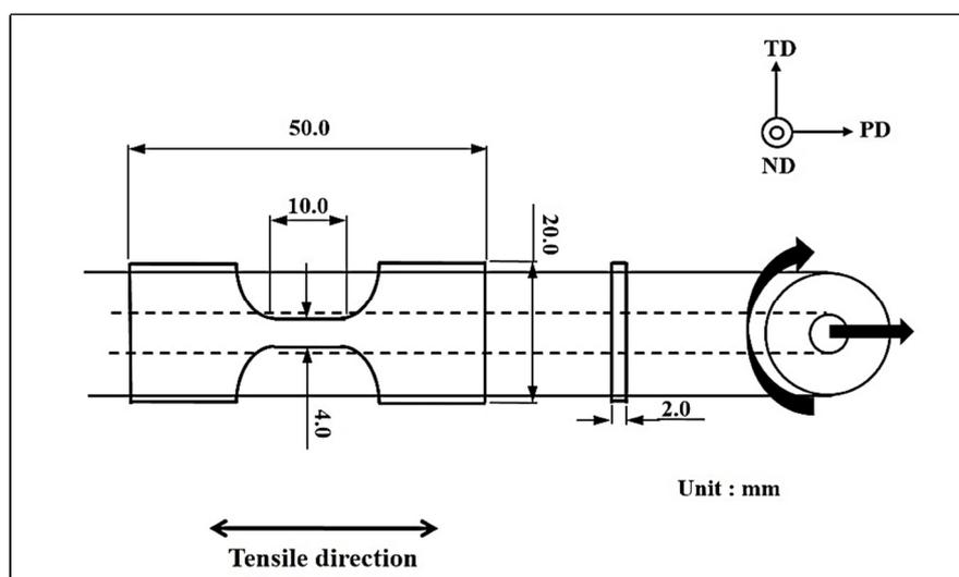
**Figure 2.** Schematic illustration of the tensile specimen (FSP). Processing direction: PD; normal direction: ND; transverse direction: TD.
