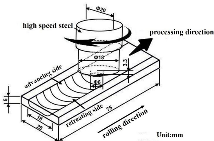
Figure 1. Schematic illustration of the friction stir process (FSP).
