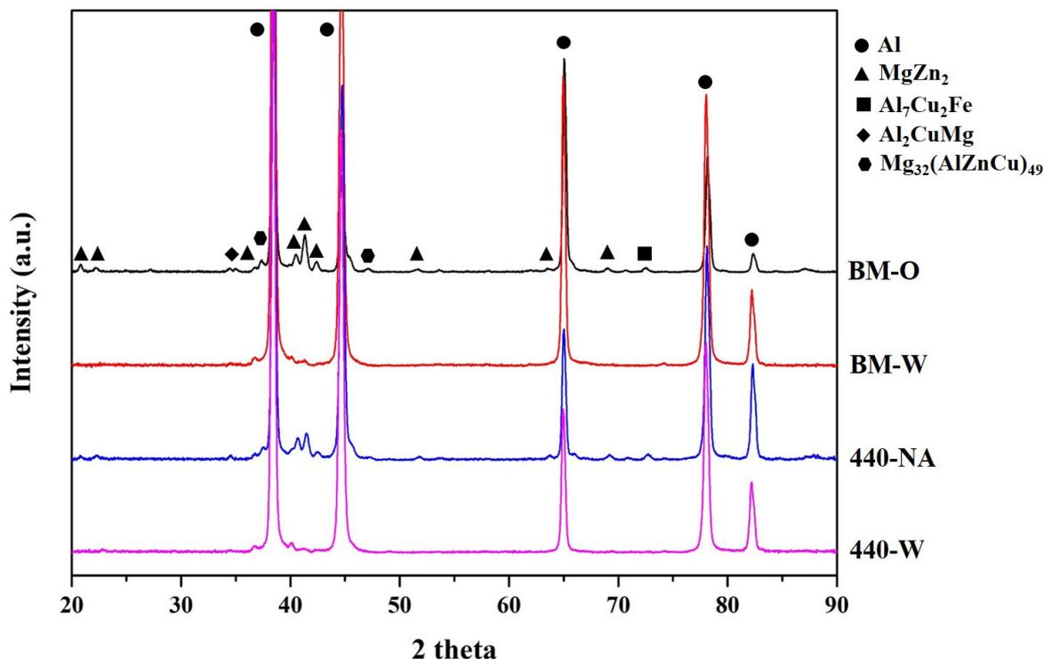
**Figure 7.** The XRD analysis of 7075 aluminum alloy after FSP and various heat treatments.
