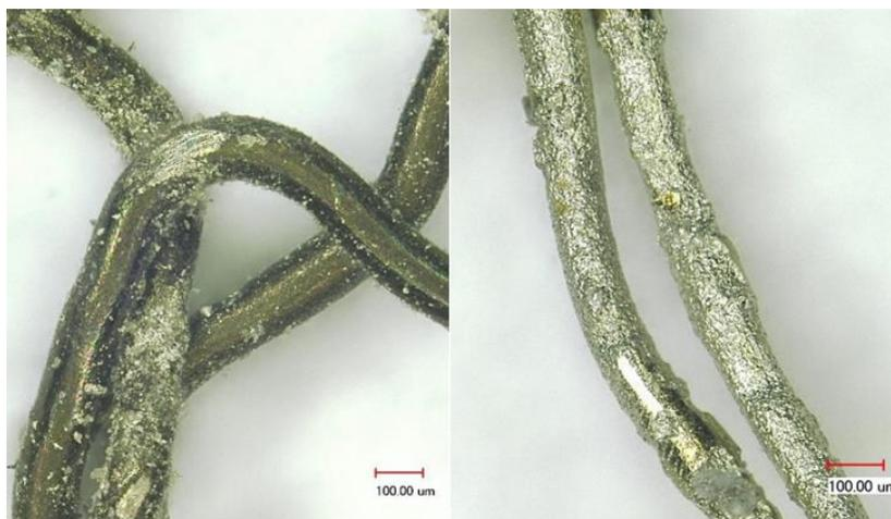
**Figure 7.** Silver cementation on nickel threads.
