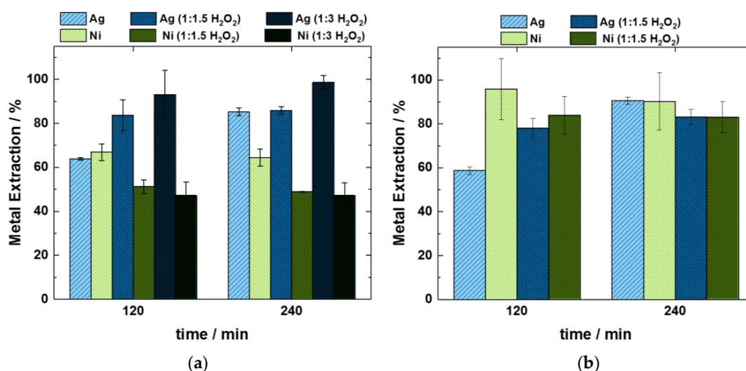
**Figure 4.** Recovery rate for silver and nickel for leaching trials with (a) 5% HNO<sub>3</sub> and (b) 10% HNO<sub>3</sub>.
