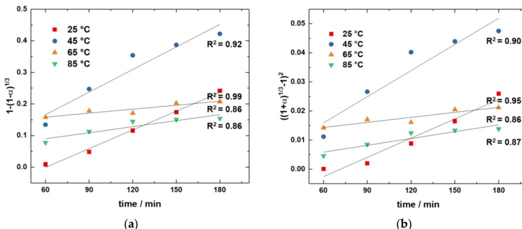
**Figure 6.** The relationship between (a)  $1 - (1 - \alpha)^{1/3}$  (reaction-controlled) and (b)  $((1 + \alpha)^{1/3} - 1)^2$  (diffusion-controlled) and the time for silver leaching at various temperatures.
