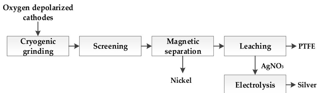
**Figure 1.** Schematic procedure for recycling silver from oxygen-depolarized cathodes (ODCs).
