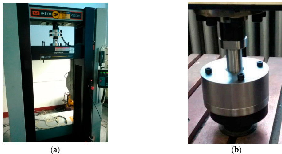
Figure 9. (a) Instron 5500R load frame device [29]; (b) Spherical indenter.
