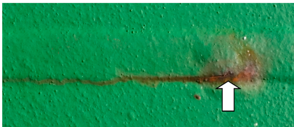
Figure 1. Crack at the weld toe.
