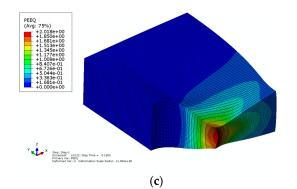
**Figure 7.** Distribution maps of equivalent plastic strain  $\varepsilon_e^{pl}$  for subsequent nominal strain levels: (**a**)  $\varepsilon = 0.09$ , (**b**)  $\varepsilon = 0.15$  and (**c**)  $\varepsilon = 0.18$ .
