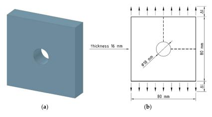
**Figure 2.** (a) View of the structural component with the defect in the form of a central hole, which was the subject of simulations. (b) Geometry and load of the model of the analysed component.
