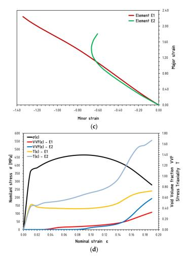
**Figure 10.** (a) Designation of finite elements E1 and E2 in the analysed numerical model. (b) Diagram of changes of equivalent plastic strain  $\varepsilon_e p^l$  and the *VVF* versus nominal strain  $\varepsilon$  for elements E1 and E2. (c) Plastic principal strain path for elements E1 and E2. (d) Diagram of changes of nominal strain  $\sigma$ , *VVF* and *T* values over nominal strain  $\varepsilon$  for elements E1 and E2.
