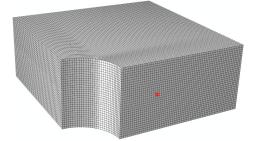
**Figure 4.** Location of the finite element, in which the most intense development of damage and the highest gradient of stress triaxiality *T* was observed.
