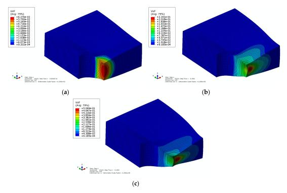
**Figure 8.** Distribution maps of the void volume fraction *VVF* for subsequent nominal strain levels: (a)  $\varepsilon = 0.09$ , (b)  $\varepsilon = 0.15$  and (c)  $\varepsilon = 0.18$ .
