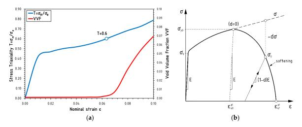
**Figure 5.** (a) Curve of changes to the stress triaxiality *T* and the void volume fraction *VVF* versus nominal strain  $\varepsilon$ . (b) Material damage model assumed for the analysis.
