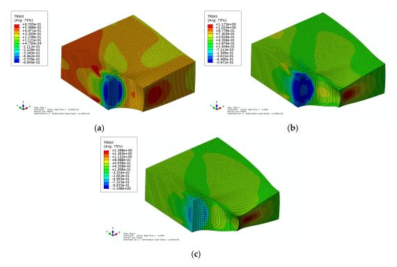
**Figure 9.** Distribution maps of stress triaxiality *T* for subsequent nominal strain levels: (a)  $\varepsilon = 0.09$ , (b)  $\varepsilon = 0.15$  and (c)  $\varepsilon = 0.18$ .
