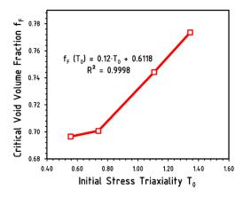
**Figure 6.** Diagram of the relationship of the critical void volume fracture  $f_F$  and the initial stress triaxiality  $T_0$  for S235JR steel [22].
