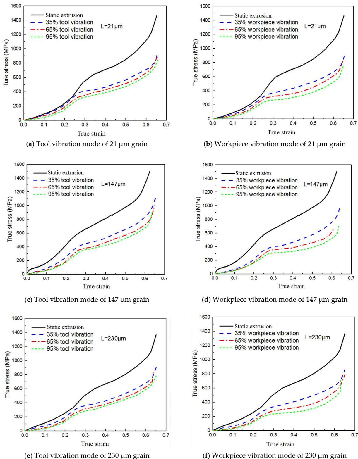
**Figure 5.** True stress and true strains with different ultrasonic power outputs.
