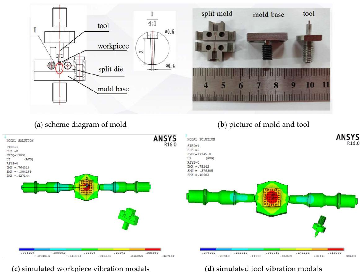
**Figure 4.** The structure of micro forming molds/tools (a,b) and the simulated ultrasonic vibration modals(c,d).
