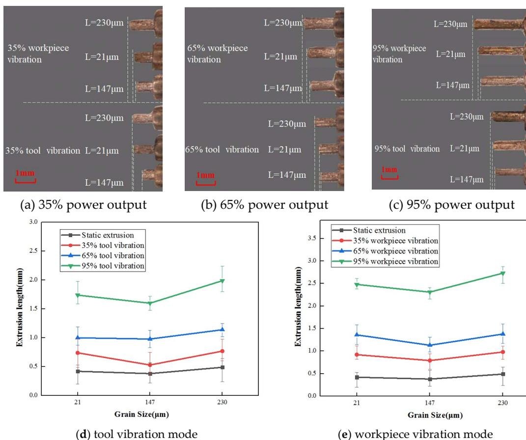
Figure 10. Micro-extrusion lengths with different initial grain size.
