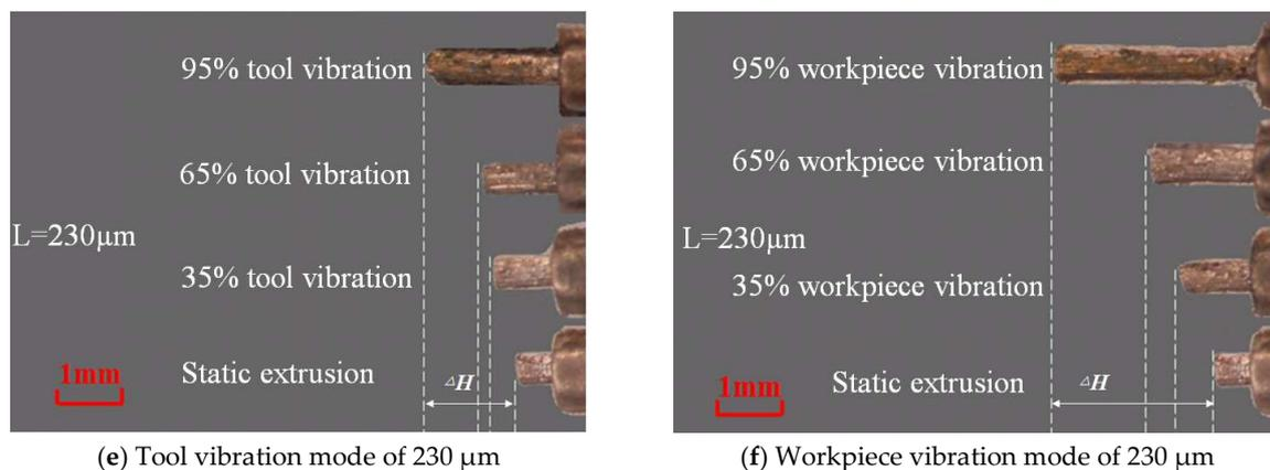
Figure 7. Micro-extrusion lengths with different ultrasonic power outputs.
