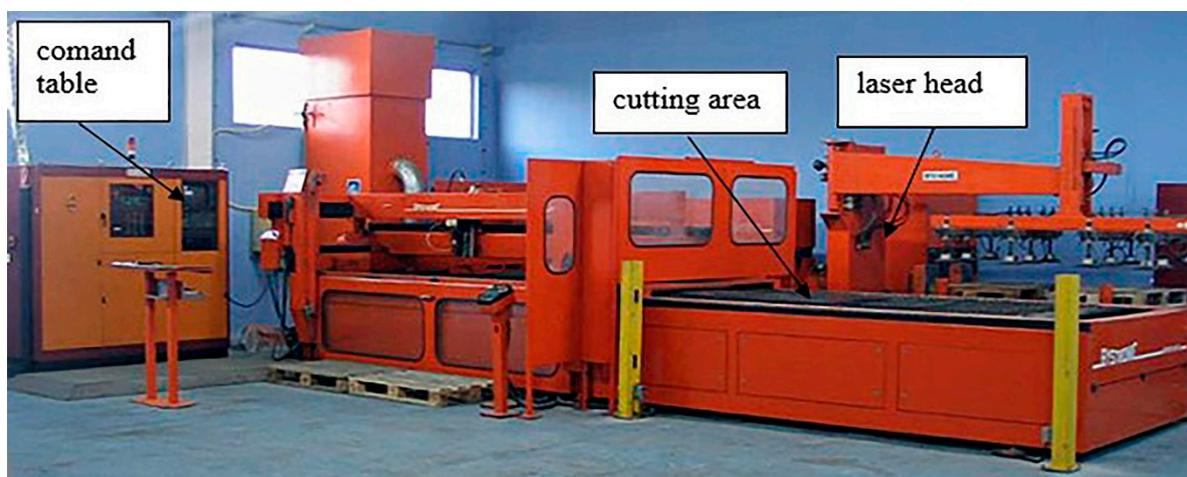
**Figure 1.** Laser cutting system BYSTAR 3015, 2.8 kW, with two tables 1500 × 3000 mm.
