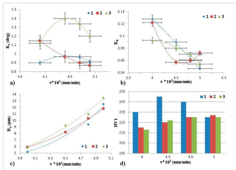
**Figure 6.** Cut quality vs. cutting speed and focus position: (a) Kerf taper, (b) Kerf deviation, (c) average roughness, and (d) microhardness. 1—material top, 2—material bottom, 3—0.5 mm in front of material.
