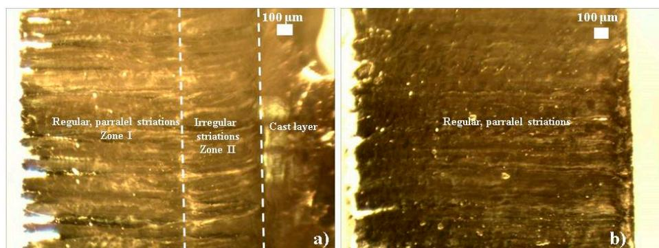
**Figure 7.** Appearance of the laser cut on Nimonic surface: (a) before optimization; (b) after optimization, taken by an optical microscope (magnification  $30\times$ ).
