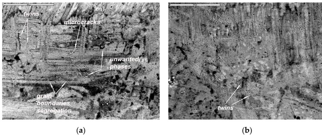
**Figure 9.** Microstructure of the cut material, shown by scanning electron microscopy: (a) before optimization; (b) after optimization. Bars in the upper left corner denote 50  $\mu\text{m}$ .
