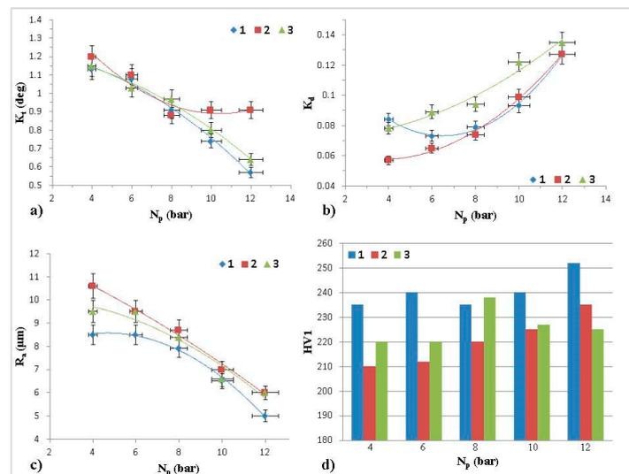
**Figure 4.** Cut quality vs. nitrogen pressure and focus position: (a) Kerf taper, (b) Kerf deviation, (c) average roughness, and (d) microhardness. 1—material top, 2—material bottom, 3—0.5 mm in front of material.
