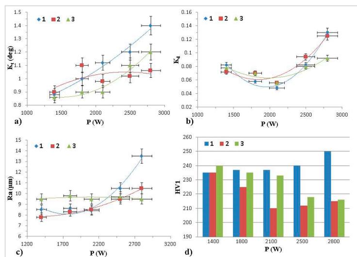
**Figure 5.** Cut quality vs. laser power and focus position: (a) Kerf taper, (b) Kerf deviation, (c) average roughness, and (d) microhardness. 1—material top, 2—material bottom, 3—0.5 mm in front of material.
