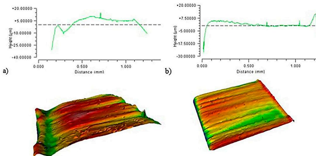
**Figure 8.** 2D profile and 3D map of the cutting area obtained by: (a) nonoptimized parameters, (b) optimized parameters.
