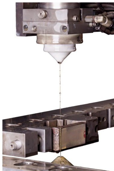
Figure 6. Method of clamping specimen 1 for wire EDM cutting.
