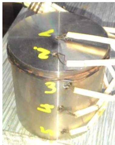
Figure 12. Temperature measurement setup.
