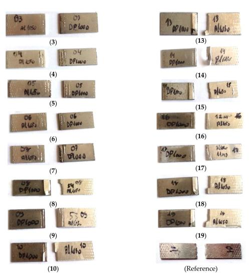
Figure 10. Samples after tensile testing.
